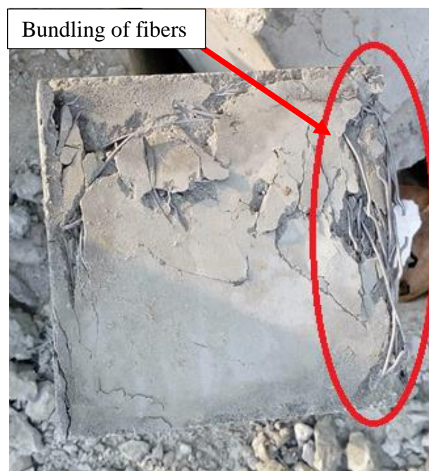
Figure 5. 6: Bundling of long hooked fibers at the corner of the cubical specimen.
