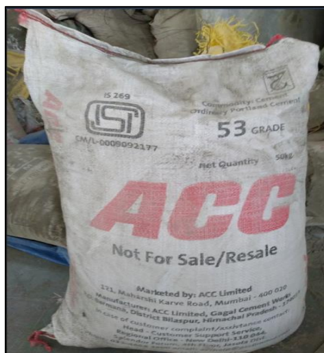
Figure 3. 1: 53 Grade OPC cement used in the present study.
