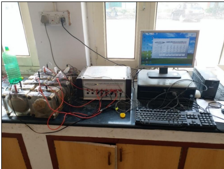
Figure 3. 16: Whole arrangement and testing during RCPT.
