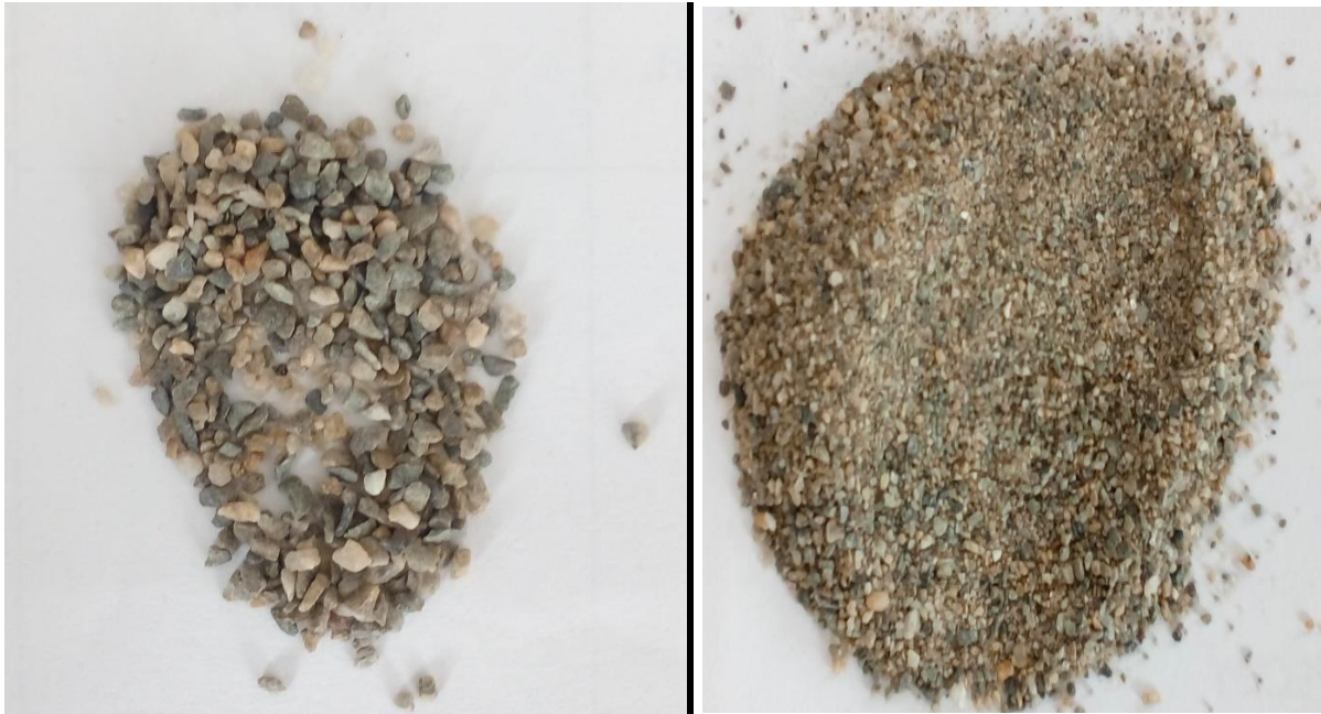
Figure 3. 3: Natural sand graded as Indian standard sand (A) Grade II (B) Grade III.
