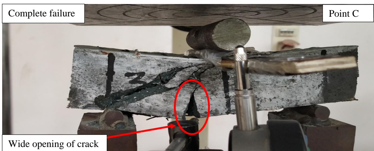
Figure 5. 12: Complete failure (Point C) of the HPHFRC (NS) beam.
