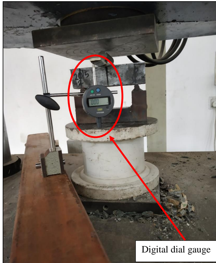
Figure 3. 12: Arrangement and testing of the flexural beam.
