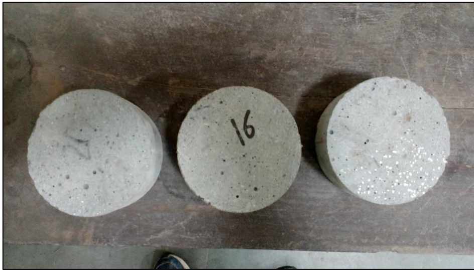
Figure 3. 15: 50 mm length cylindrical slice of 100 mm diameter for RCPT.
