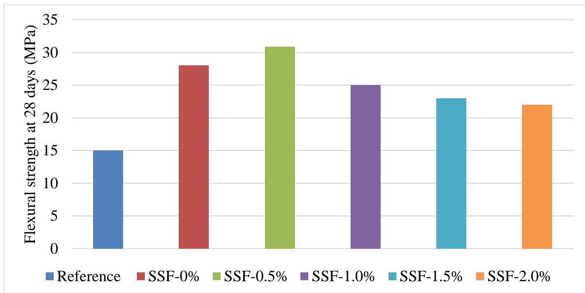
Figure 2. 13: Flexural strength of the mixes with straight and hooked steel fibers (Reference: UHPFRC without fibers) (Yu R. et al. 2015).
