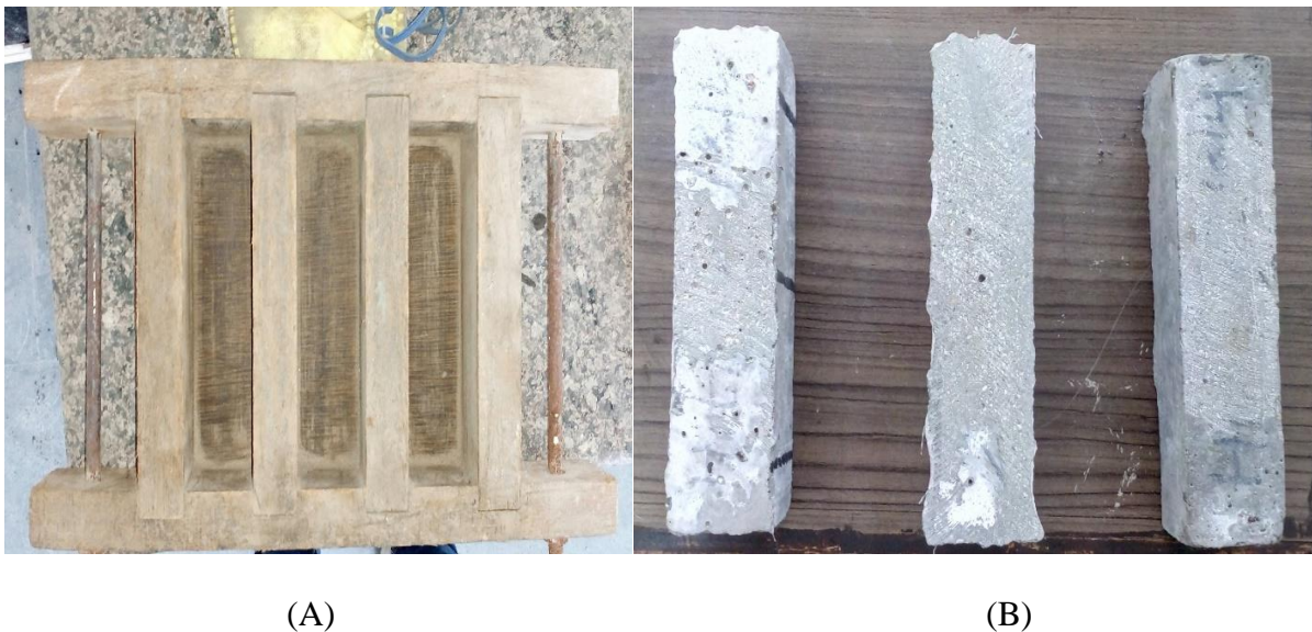
Figure 3. 11: (A) Mould for flexure specimen (B) Casted flexure specimens.
