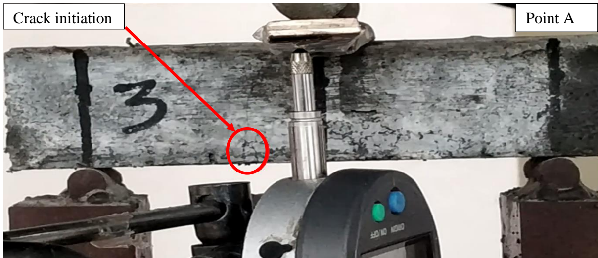
Figure 5. 10: Crack initiation (Point A) in the HPHFRC (NS) beam.
