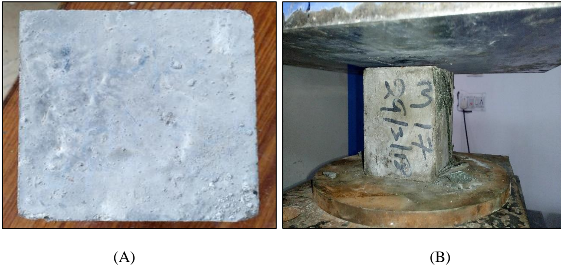
Figure 3. 9: (A) 70.6 mm cubical specimen (B) Testing of cube specimen in CTM.
