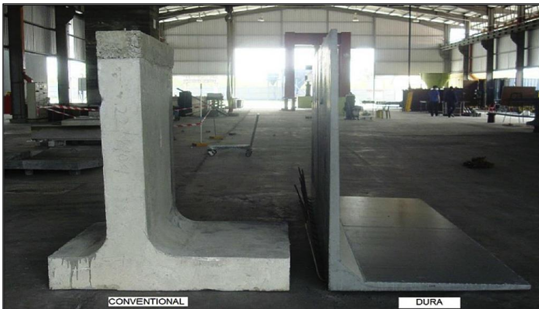
Figure 1. 4: Sectional dimensions of an L-shaped wall, built by conventional concrete and UHPFRC ( Lei et al. 2012 ).
