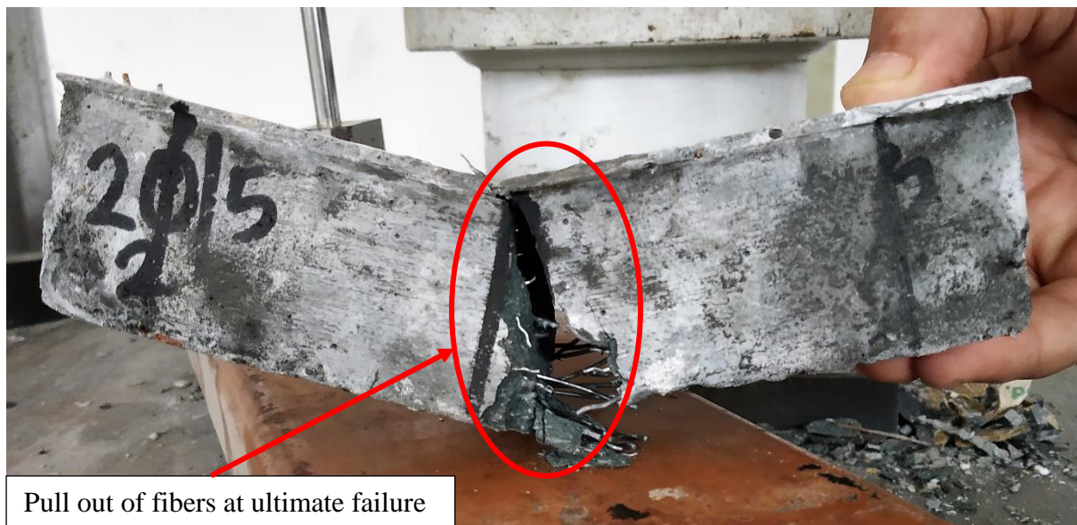
Figure 5. 13: Pull out of the fibers at very large deflection.
