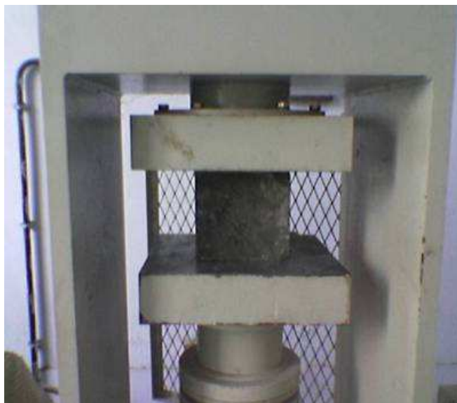
Plate 3.2 Photograph of cube placed on anvil of ACTM for compressive strength test
