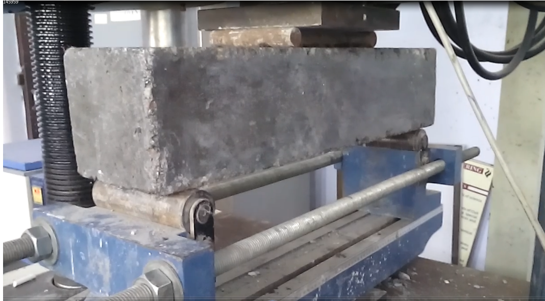
Fig. 3.7: Flexural Strength Testing of Specimen under UTM
