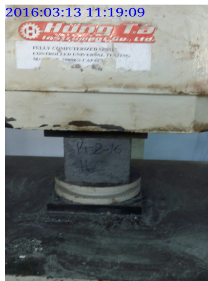
Fig. 3.3: Compressive Strength Testing of Cube under UTM
