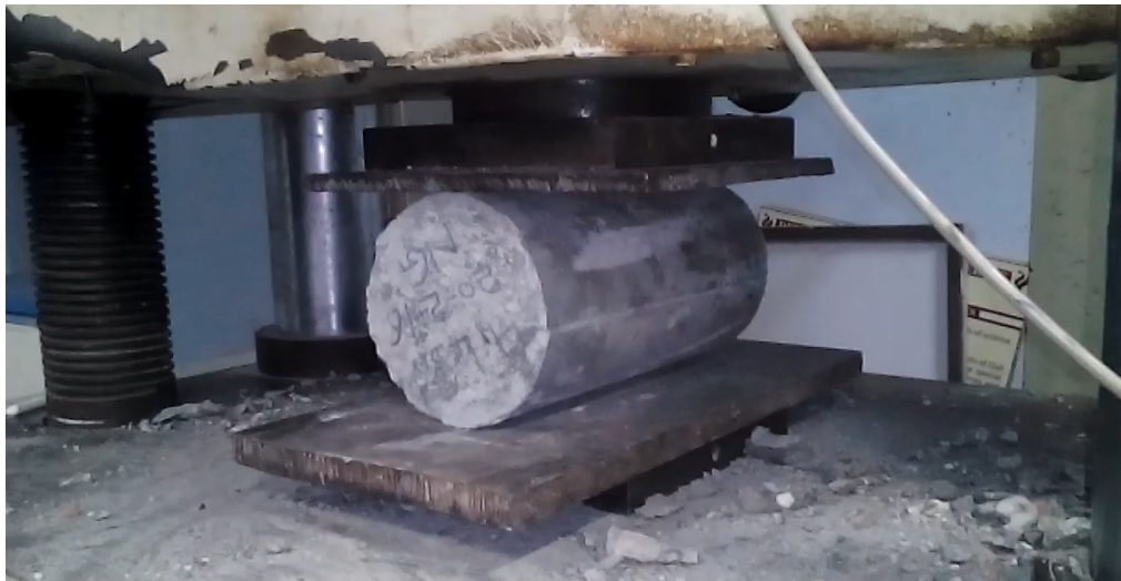
Fig. 3.5: Split Tensile Strength Testing of Cylinder under UTM
