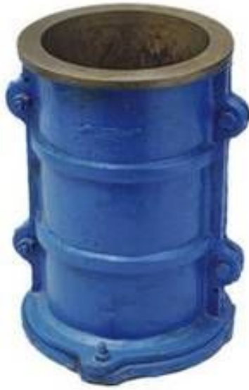
Fig. 3.4: Cylinder Specimens of Size 150mm (diameter) x 300mm for split tensile strength testing.
