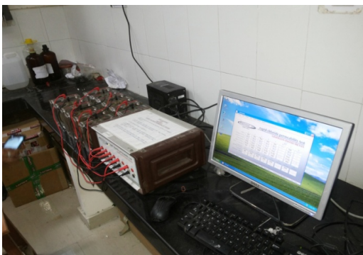
Fig.3.13: Rapid Chloride Permeability Test Setup
