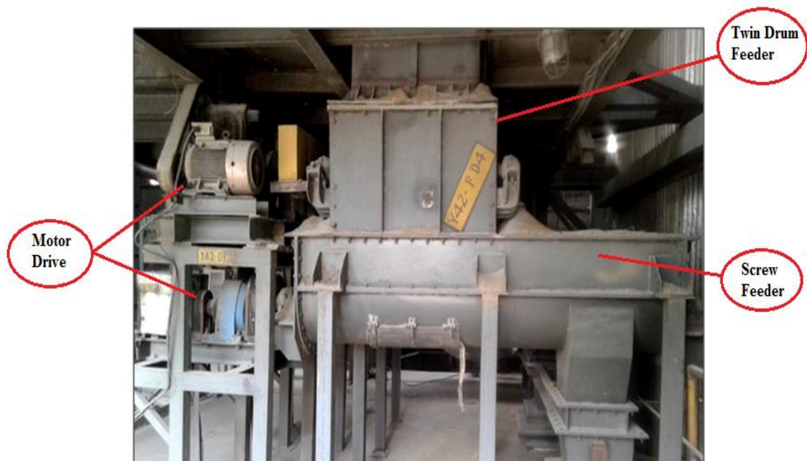
Fig. 3.12: Twin drum feeder and screw feeder
