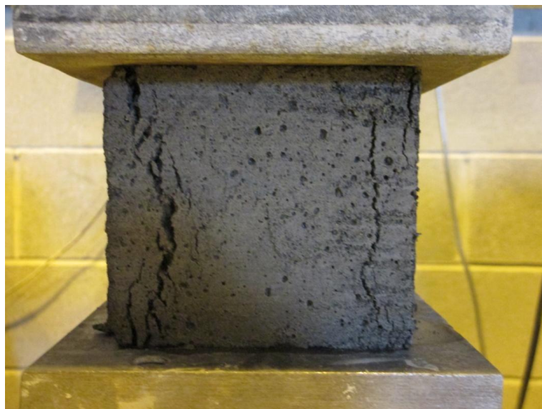
Plate 5.19 - Rough surface and cracking pattern for mix L5
