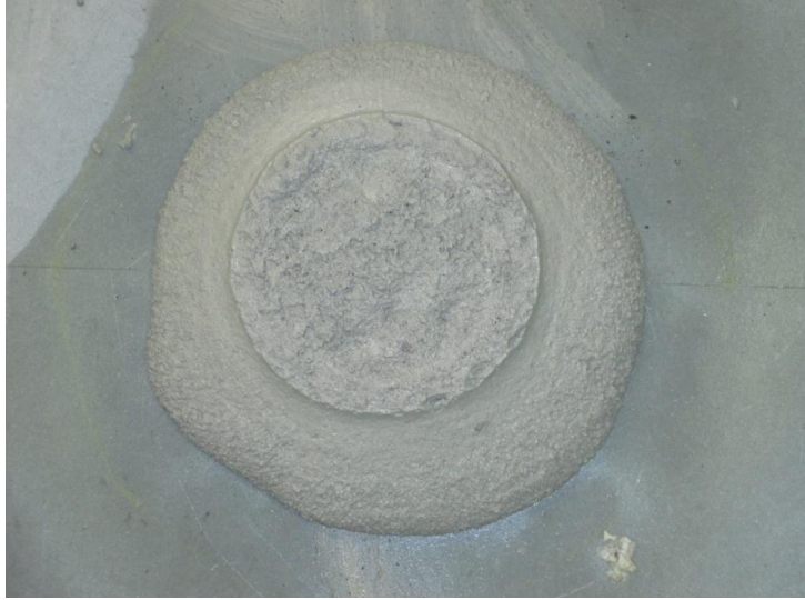
Plate 5.9 - Slump collapse mix L0
