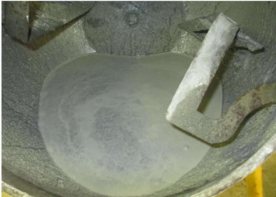
Plate 5.14 - Water on the surface in the drum mixer for mix L5
