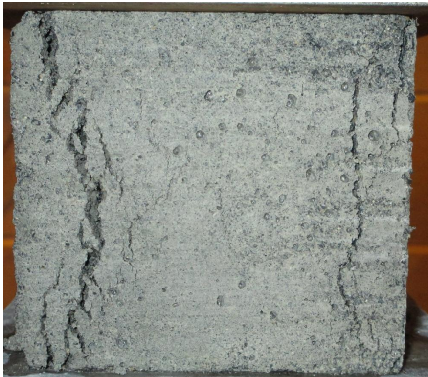
Plate 4.1 - Rough surface of cube specimen C1 after cracking
