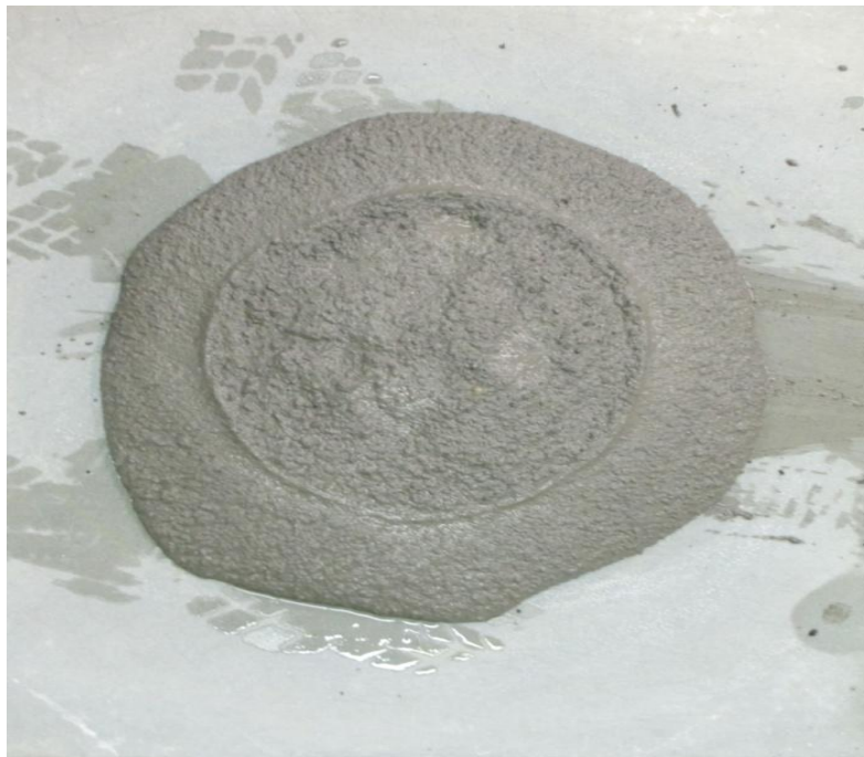
Plate 5.2 - Cone lifted for flow test (F1)
