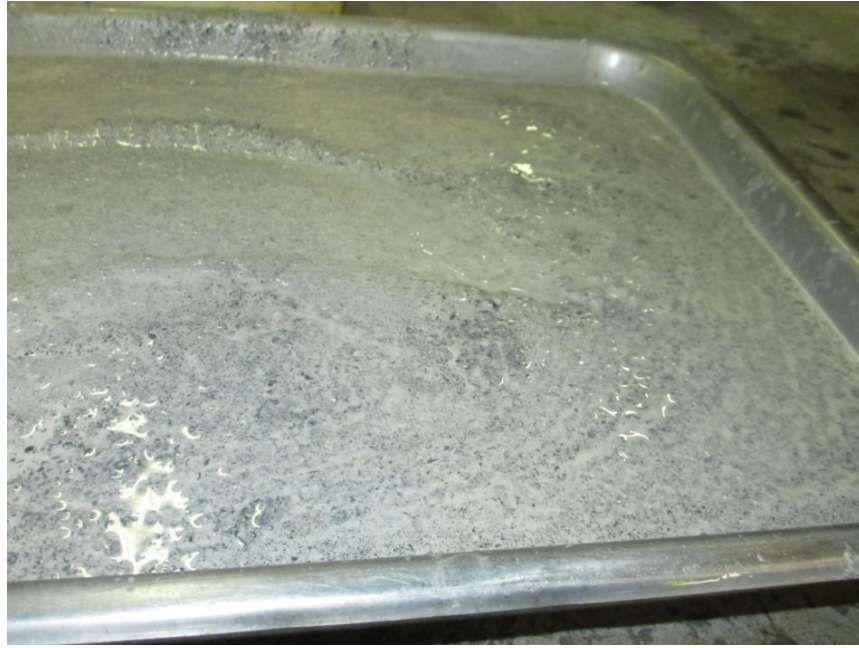
Plate 5.13 - Unmixed water in mix L4
