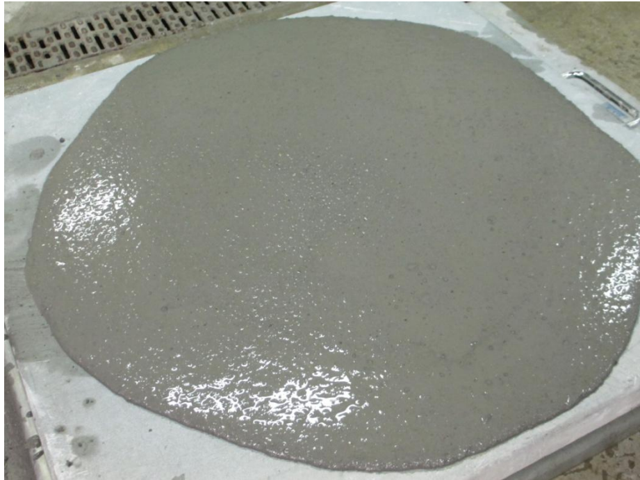
Plate 5.3 – 670mm flow diameter of mix F1
