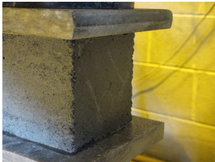
Plate 5.20 - Rough edges of 7-day cube for mix F5
