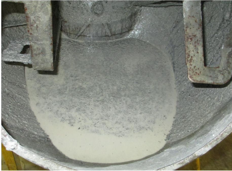
Plate 5.17 – Sand settled in the drum mixer for mix L7
