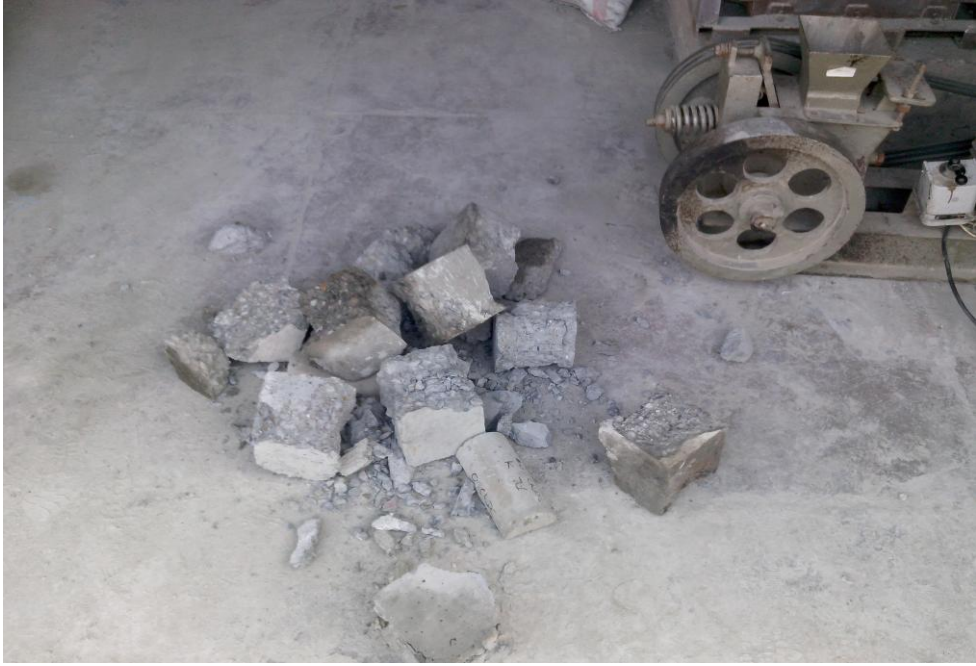
Plate 3.1: Waste concrete rubble for obtaining RCA
