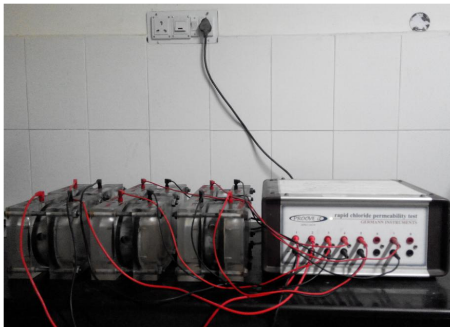
Plate 3.7: Rapid chloride permeability test
