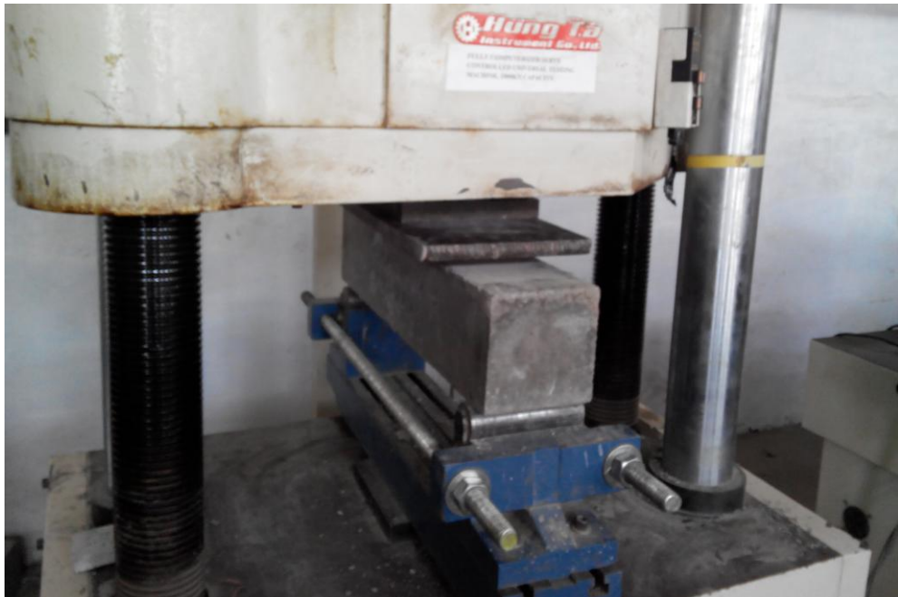
Plate 3.5: Testing for flexural strength
