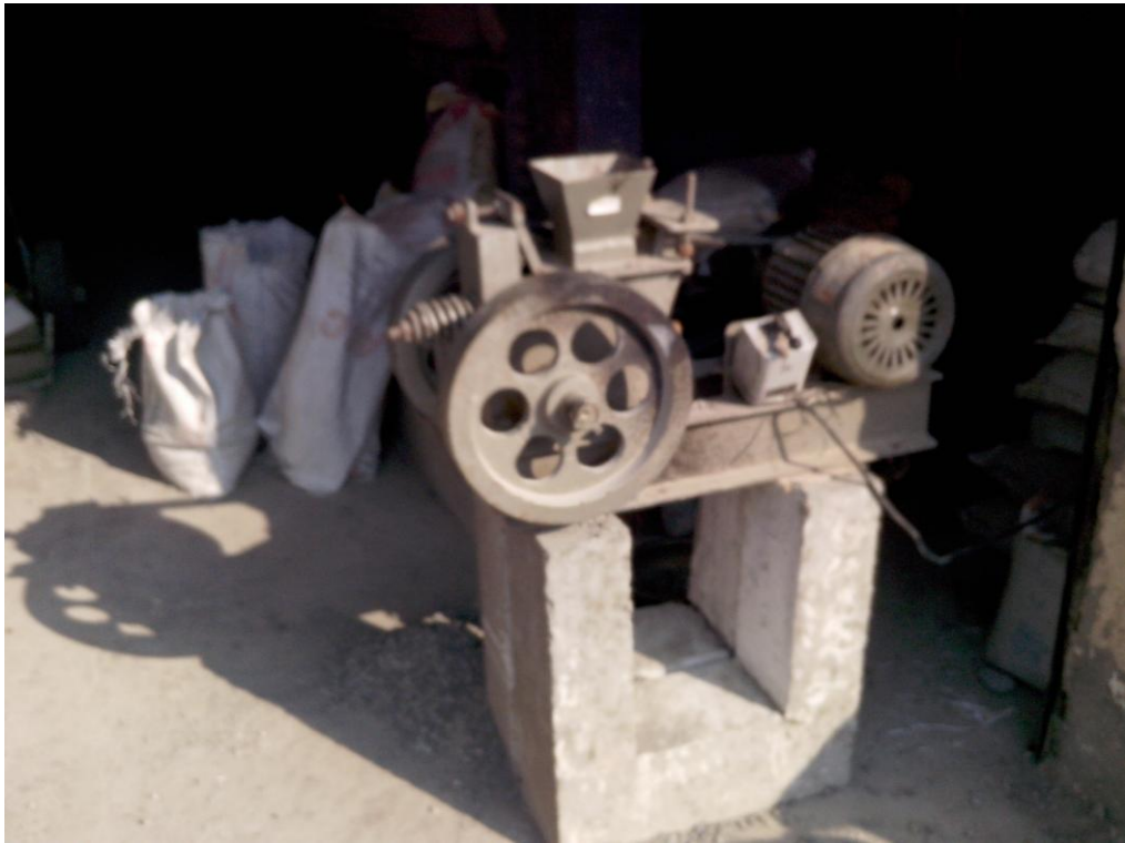
Plate 3.2: Jaw crusher to obtain RCA
