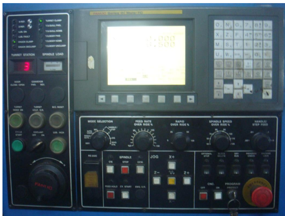
Figure 4.2: shows the Fanuc controller and panel from where the programming is done and all parameters are controlled
