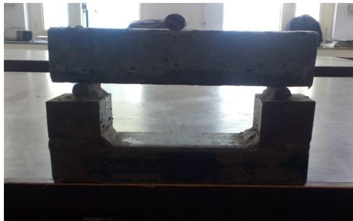
Fig 3. 16: Flexural Strength Test Arrangement (actual)
