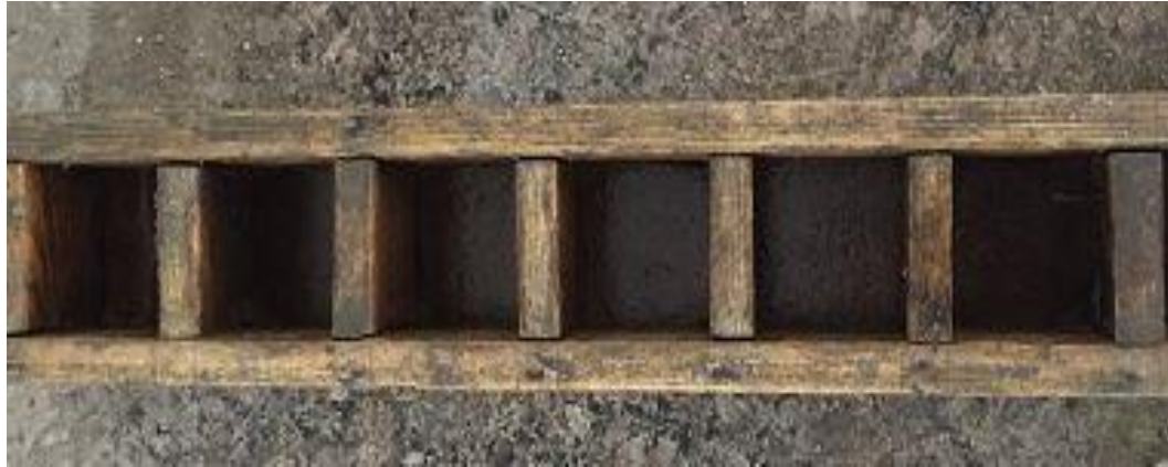
Fig 3. 23:Moulds of Cubes of Size 50mm*50mm*50mm
