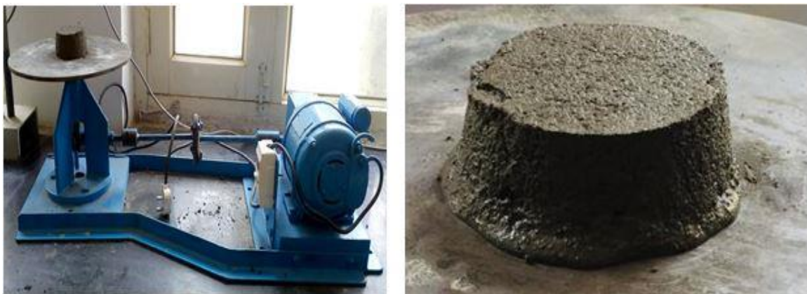
Fig 3. 5:Flow Table and Flow (Spread) in Mortar on Flow Table
