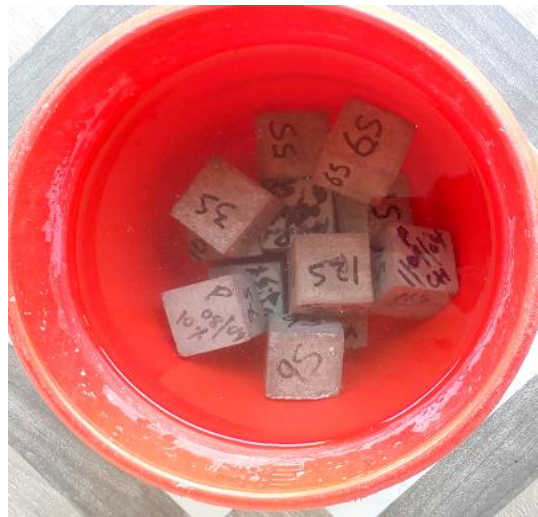
Fig 3. 25:Immersion of Samples in 14% Solution of Sodium Sulphate Decahydrate
