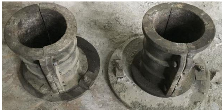
Fig 3. 30:Moulds of Cylinder of 100mm dia. and 200mm height
