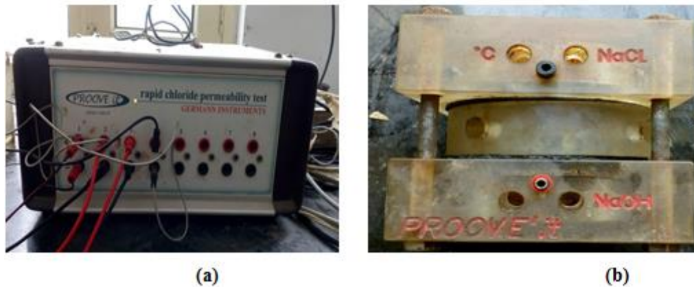
Fig 3. 34: (a) PROOVE'it Microprocessor Power Supply Unit and (b) PROOVE'it Cell
