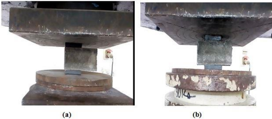
Fig 3. 12: Different Arrangements of Bearing Plates on UTM
