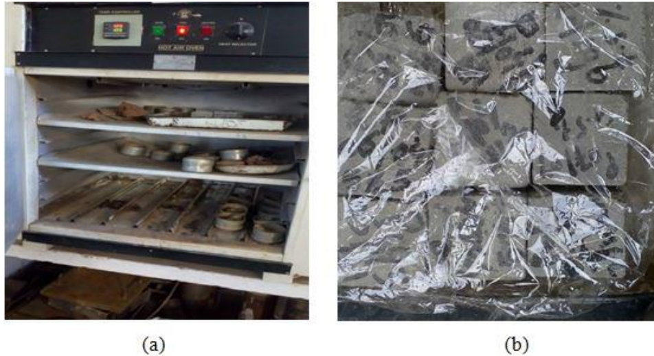
Fig 3. 20:(a) Hot Air Oven and (b) Cubes Protected from Humid Atmosphere
