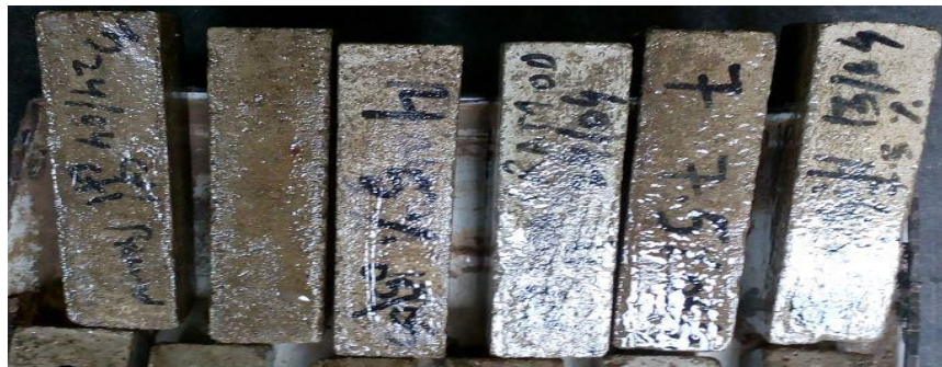
Fig 3. 10:Prisms with Epoxy Coating
