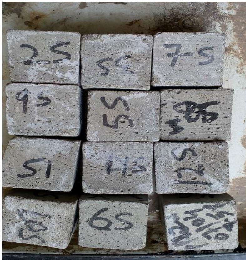
Fig 3. 29:Physical Appearance of Mortar Treated with Sodium Sulphate solution
