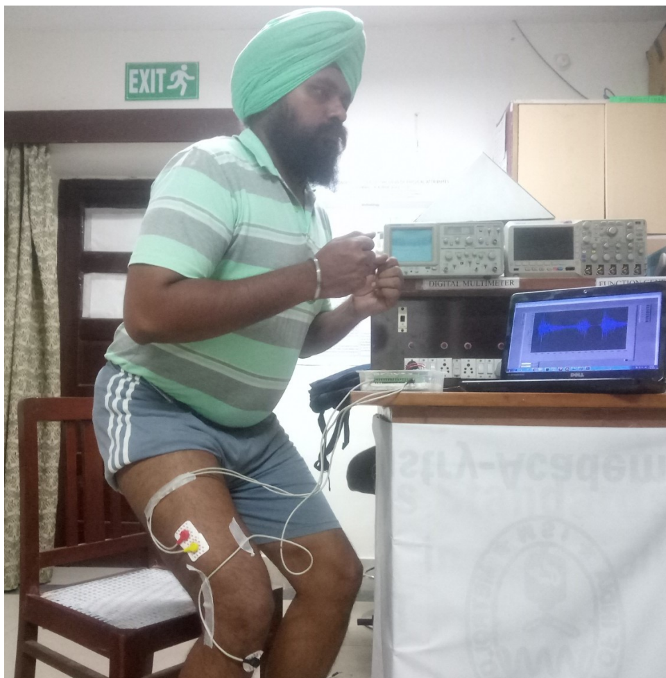
FIGURE 3.13: Setup for recording SEMG signal during standing up/ sitting down from/on a chair
