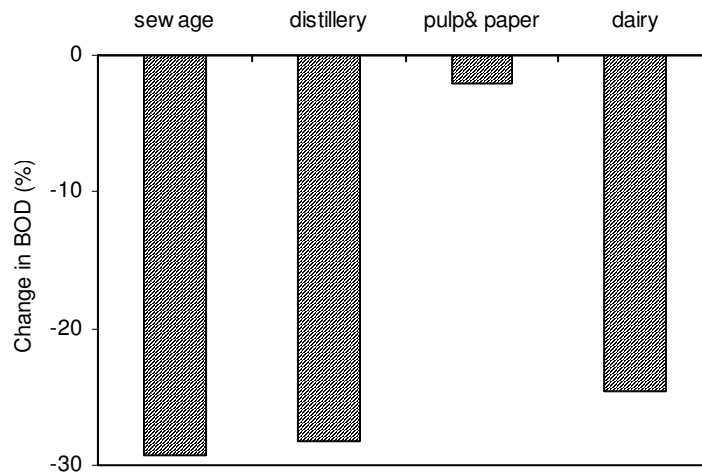
Figure 3.2 Bars of change in BOD in presence of nickel ions using different types of seed
