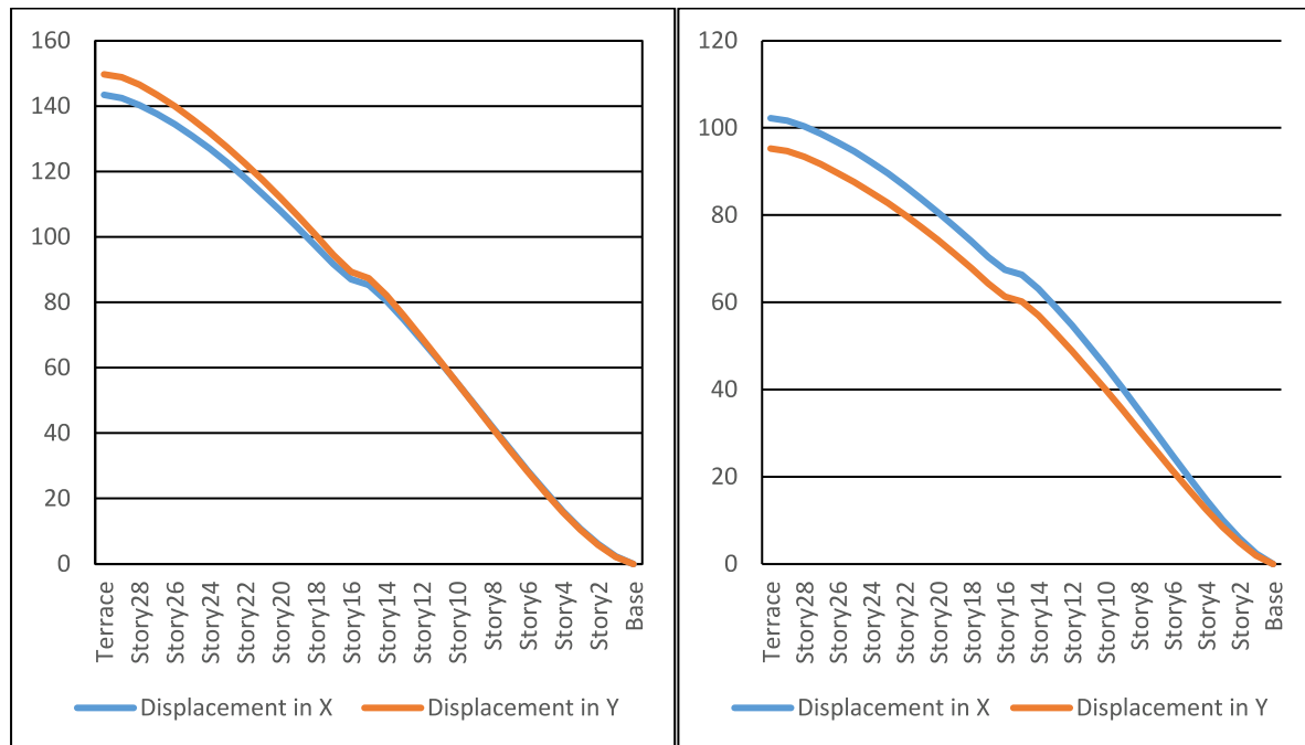
Figure 5. 6 Linear Static and Response Spectrum Analysis Results in X and Y Directions
