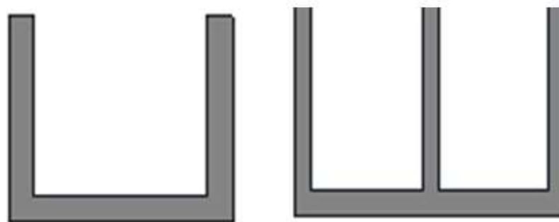
Figure 1. 5 U & W Shaped Shear Walls
