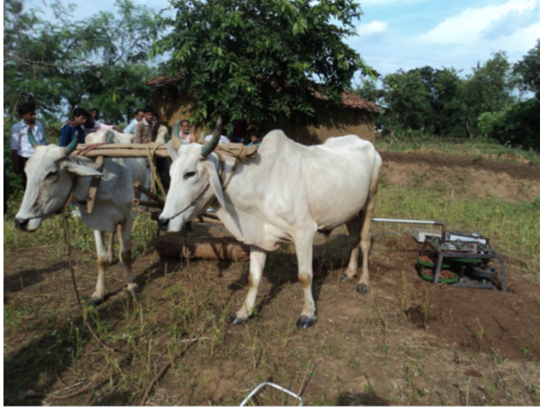
Figure 3-1: Bull Powered Generator
