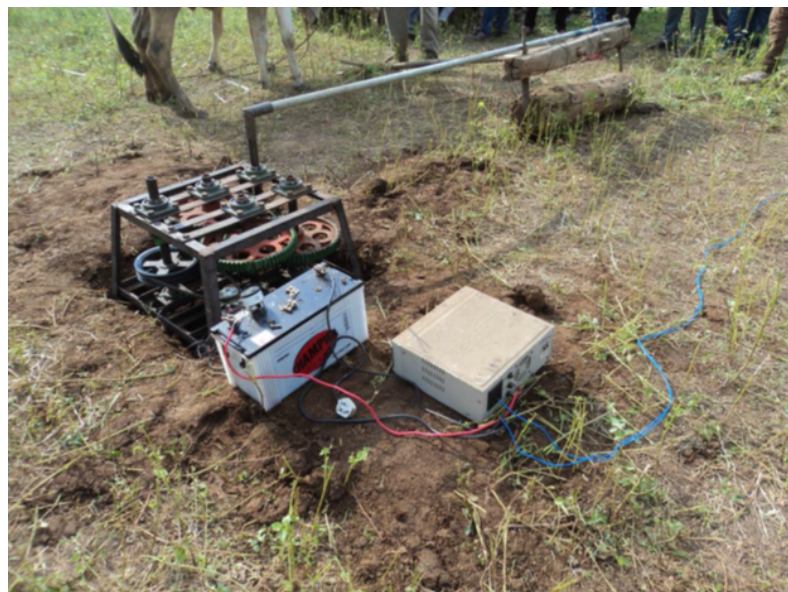
Figure 3-2: Components used in Bull Powered Generator
