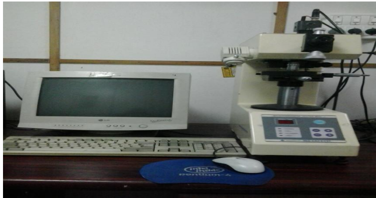
Figure 3.3 MicrohardnessTester (Courtesy by: Meteorology Lab, Thapar University, Patiala)
