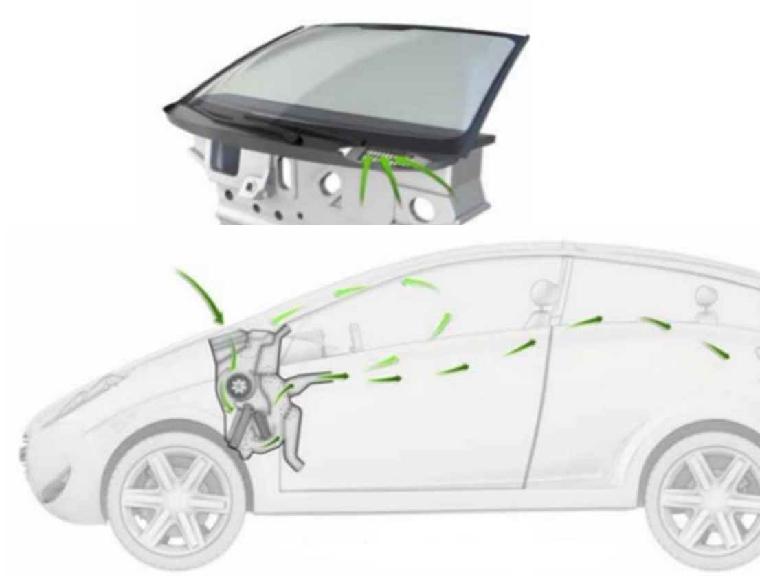
Figure 3.2: Air circulation in the car [19]
