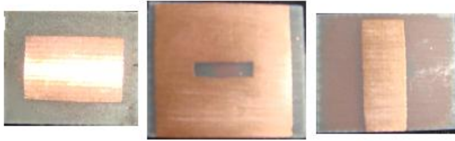
Fig 6.8 (a) Patch (b) Aperture on ground (c) Feed line of Single Band ACMA
