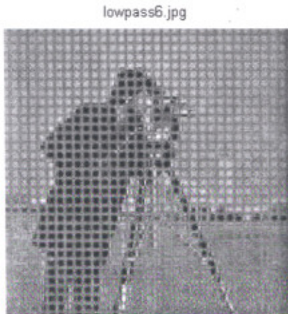
Fig6.14(c)Decompressed image ( \alpha=.9 , CR%=76.5625, RMSE=46.4480)
