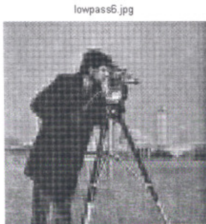
Fig6.12(c)Decompressed image ( \alpha=.97, CR\%=76.5625, RMSE=21.8548 )
