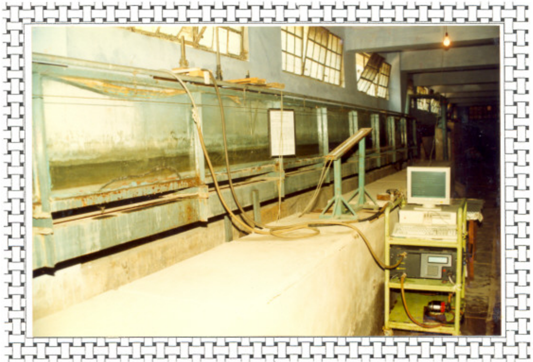
Fig. 4.8 A Photograph of Tracer Monitoring System
