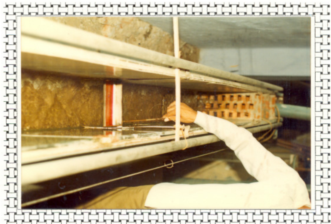
Fig. 4.3 A Photograph of Grill Wall, Wooden Suppressor and Tracer Injection Sampler
