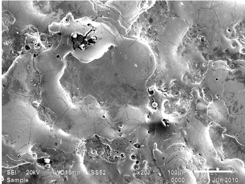
Figure 8.13: SEM micrograph at 200× of HCHCr machined with graphite electrode in copper powder mixed in EDM oil (I 5Amp, pulse on time 50µs, pulse off time 57µs)
