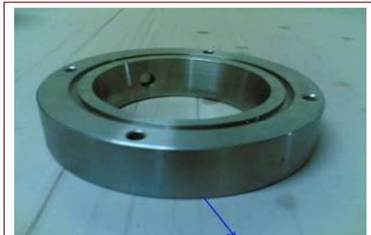
It provides space for rotation of valve
