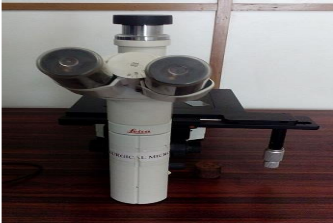
Figure 3.10 Metallurgical Microscope [Courtesy: Advanced metallurgical lab, Thapar University, Patiala]
