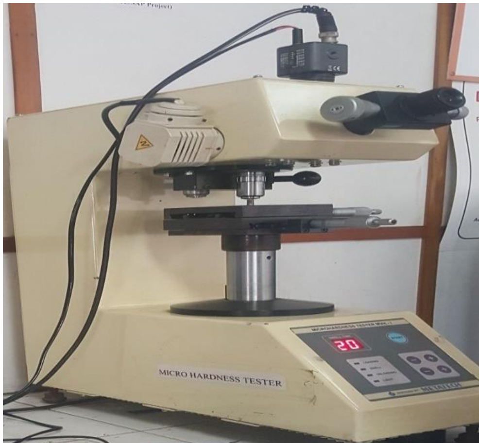
Figure 3.14 Micro-hardness tester [Photo Courtesy: Thapar university campus, Patiala]
