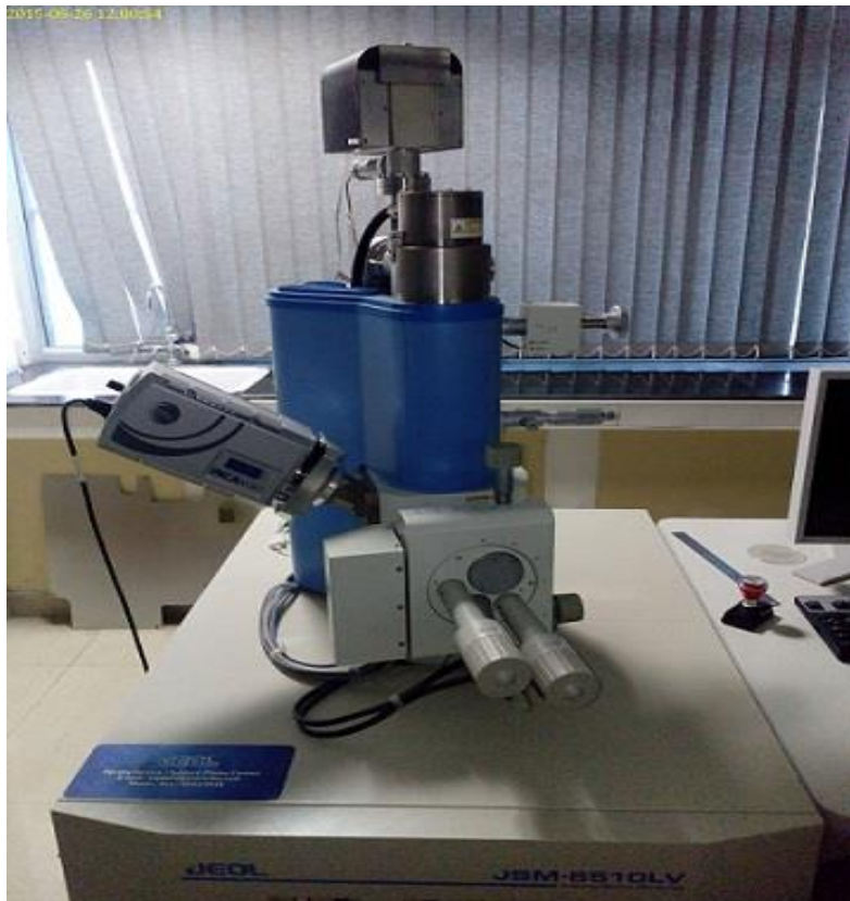
Figure 3.9 Scanning electron microscope [Photo courtesy: SAI Labs, Thapar University Campus, Patiala]
