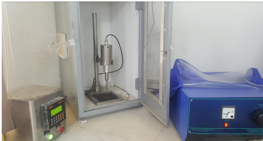
Figure 3.6 Ultrasonicator [Photo Courtesy: Thapar university campus, Patiala]
