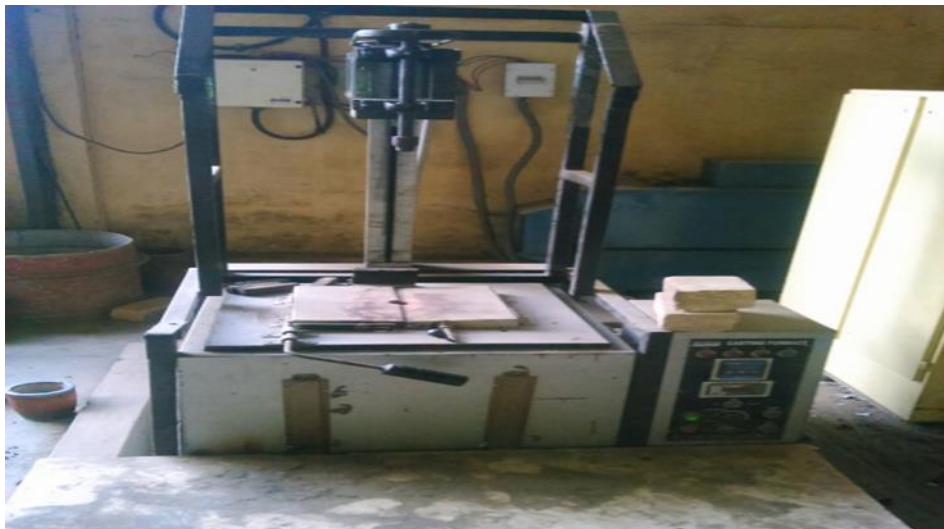
Figure 1.1 Stir Casting Furnace [Photo courtesy: Thapar university campus, Patiala]
