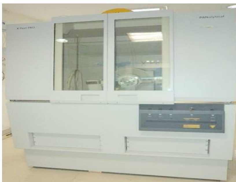
Figure 3.8 X-ray diffractometer [Photo courtesy: SAI Labs, Thapar University Campus, Patiala]
