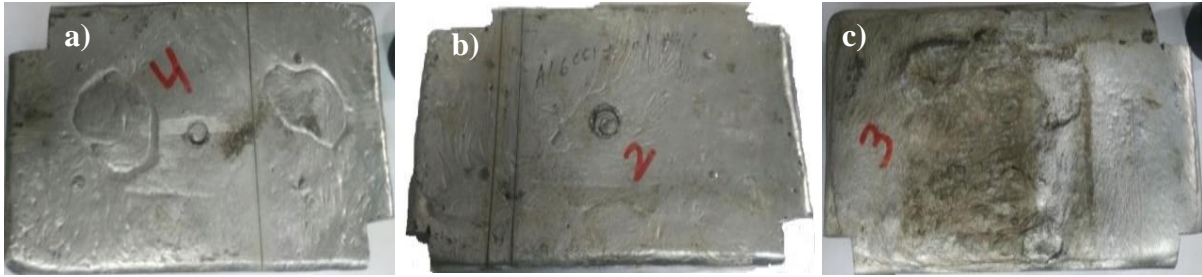
Figure 3.3 Cast composites (a) SiC 5% B 4 C 5%, (b) B 4 C 10%, (c) SiC 10% [Photo courtesy: Thapar university, Patiala]
