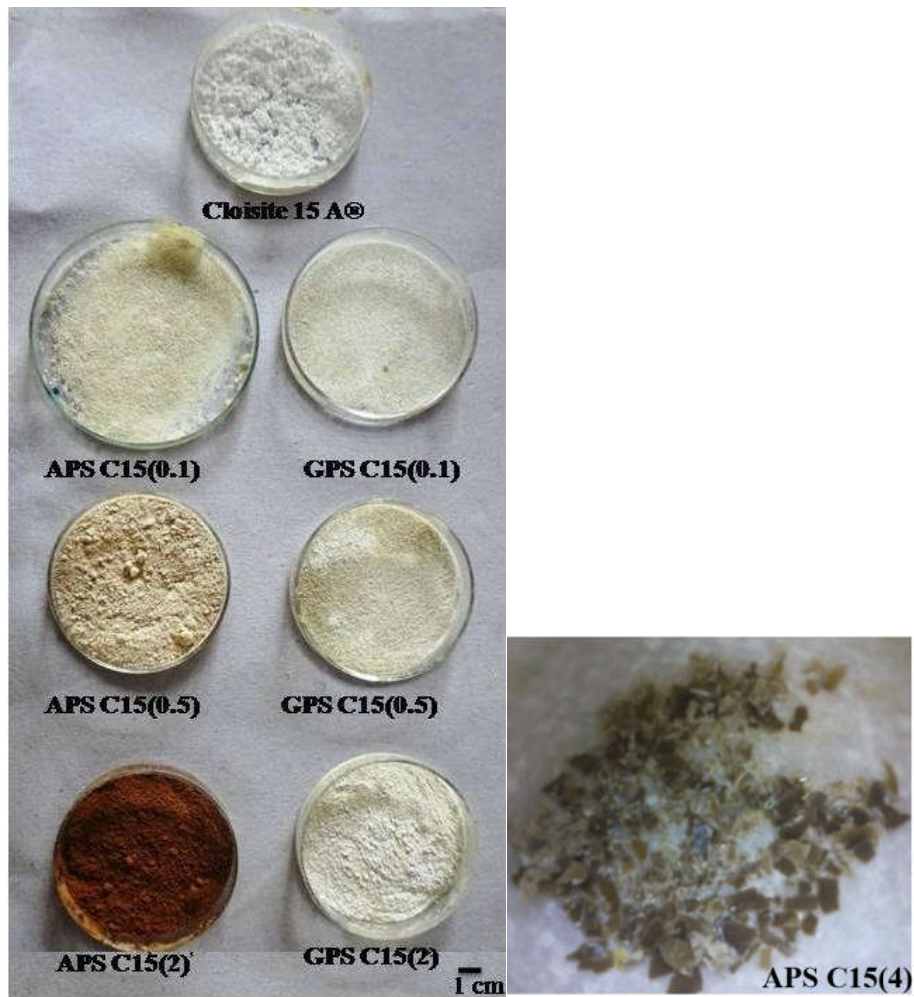
Figure 4.1 Clay minerals after silane treatment as a function of concentration of silanes in solution
