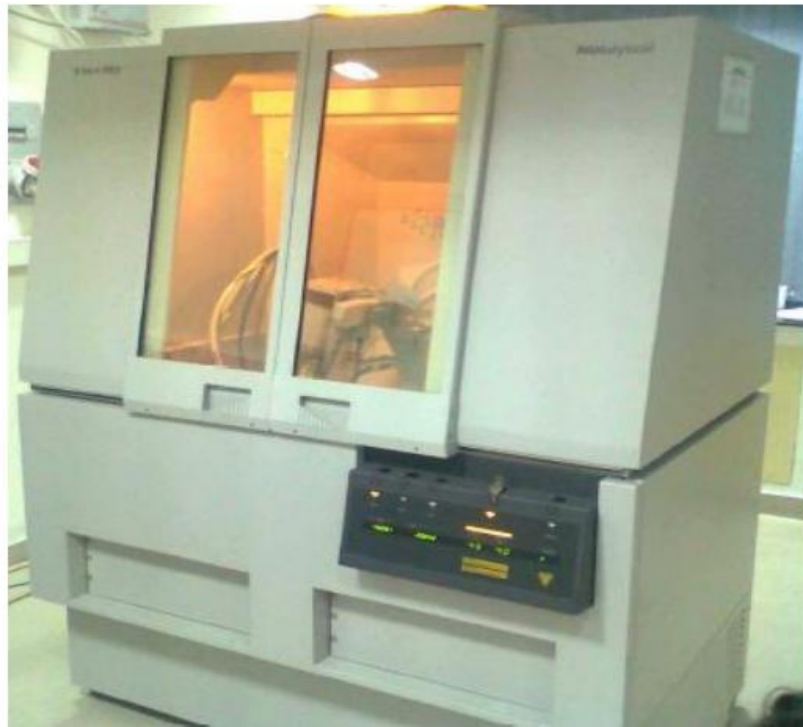
Figure 2.4: Laboratory view of X-Ray Diffraction spectrometer.
