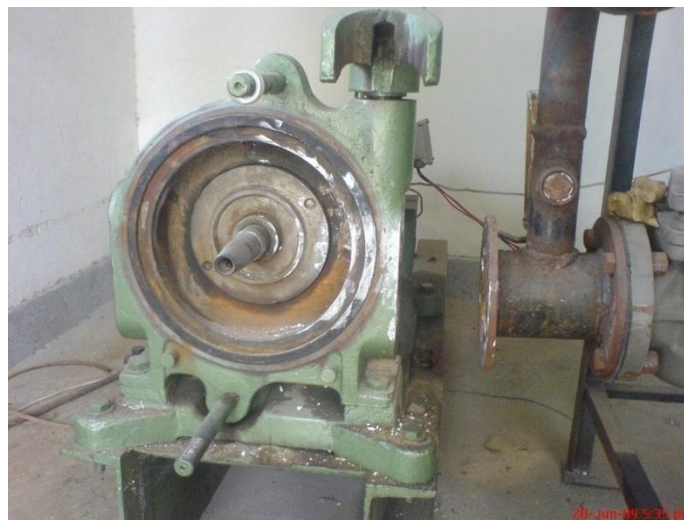
Figure 5.6 Dismantled pump for dimensioning of inlet passage
