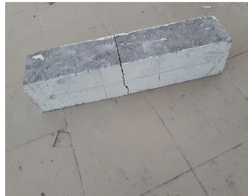
Figure 5-7 Cracks in Beam after testing
