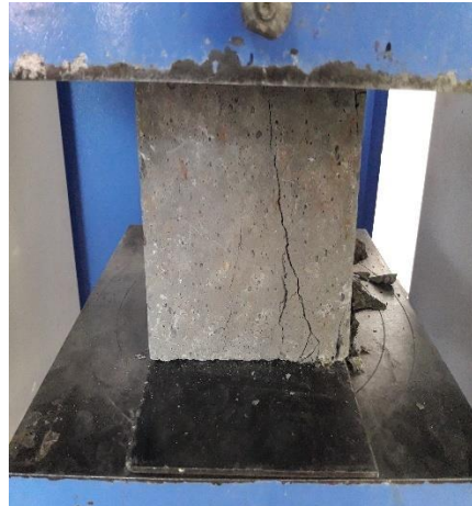
Figure 5-2 Cracks on cube after testing
