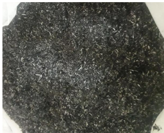
Figure 1-19 Actual picture of Rice Husk Ash used in study
