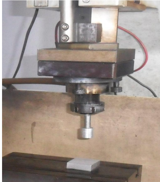
Figure 3.2: Experimental setup for EDM of Al MMCs.
