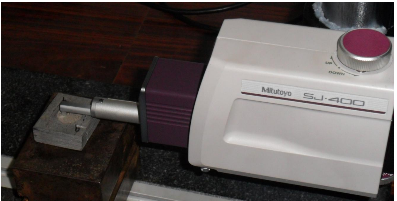
Figure 3.3: Measurement of surface Roughness using Surface roughness tester
