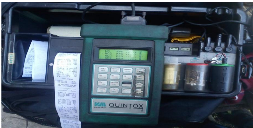
Figure 3.9: Flue gas analyzer
