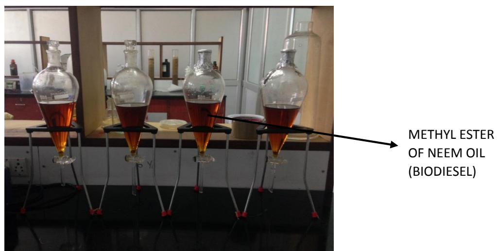
Figure 3.4: Final methyl ester of neem oil formed after the hot water washing.
