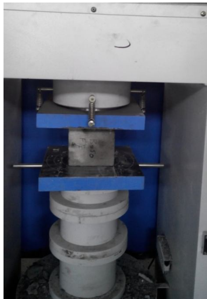
Fig 3.1 Testing for compressive strength
