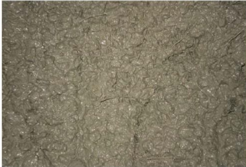
Fig 2.2 Physical appearance of fresh SFRC in the drum mixer (Ibrahim et al., 2013)
