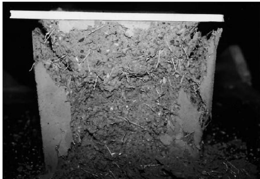
Fig 2.9 Steel Fibre distribution in the Cube of SFRC after the test of Compression Strength (Kusterle et al., 2000).
