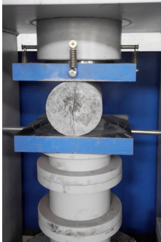
Fig 3.2 Testing for splitting tensile strength
