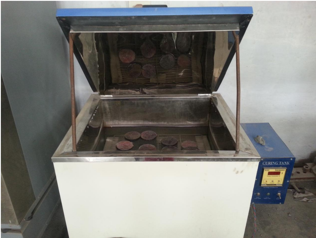
Plate 3.5 Samples boiled in curing tank at maintained temperature.
