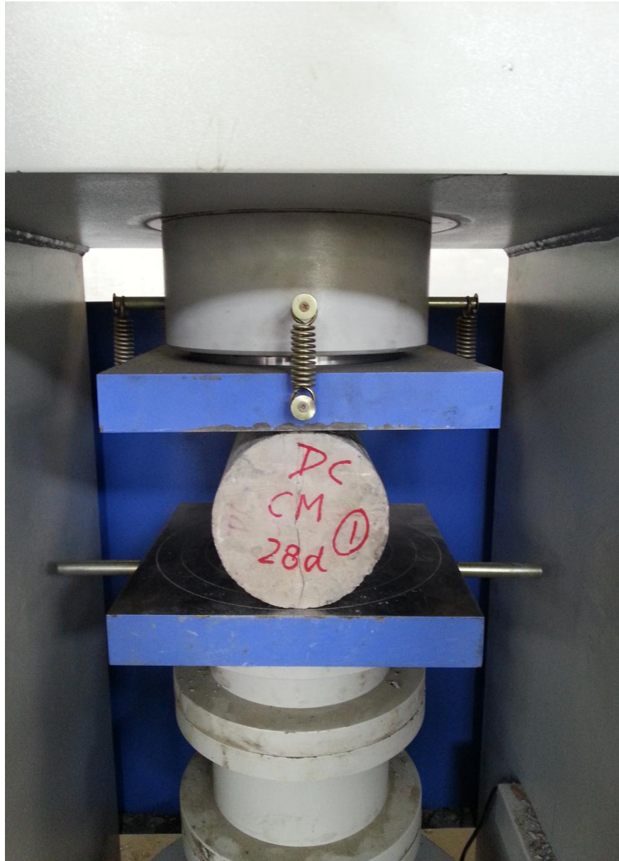
Plate 3.3: Split tensile strength machine used in this study
