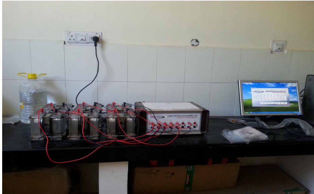
Figure 3.6: Rapid chloride permeability test set up (ASTM C 1202).
