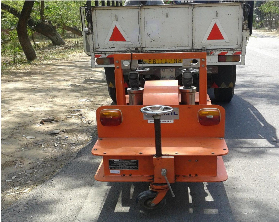
Figure 4.24: Bump Integrator Test in Progress on Section UR-03
