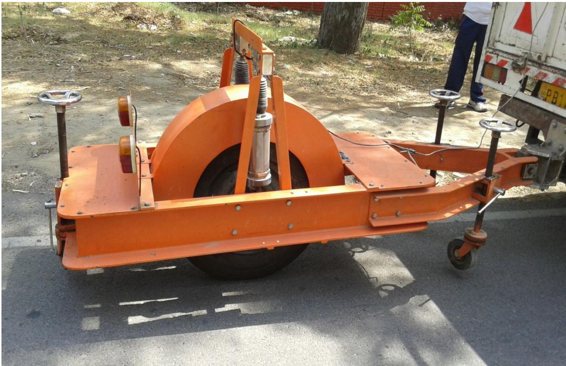
Figure 4.25: Bump Integrator Test in Progress on Section UR-04
