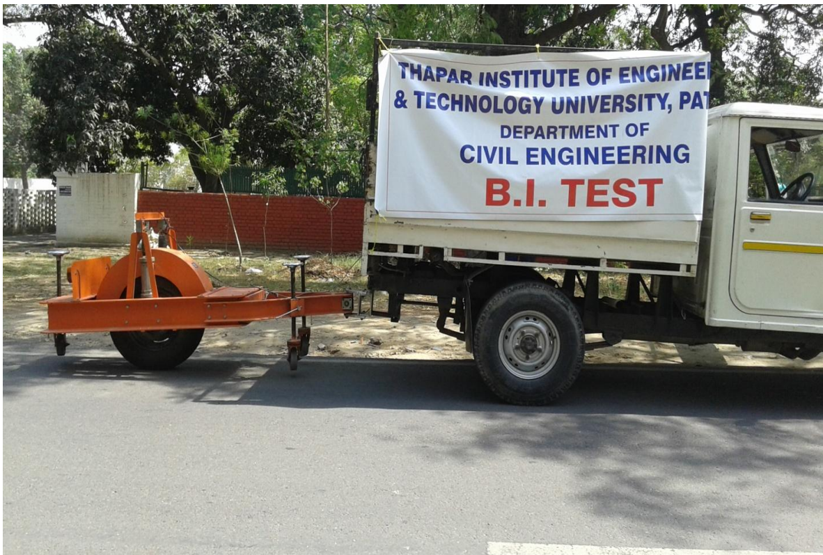
Figure 4.23: Bump Integrator Test (Roughness Test) in Progress on Section UR-03
