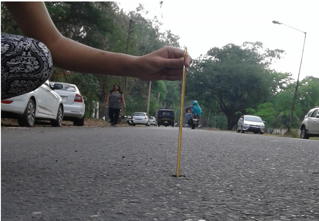
Figure 4.12: Determination of Actual Pavement Temperature on Road Section UR-03
