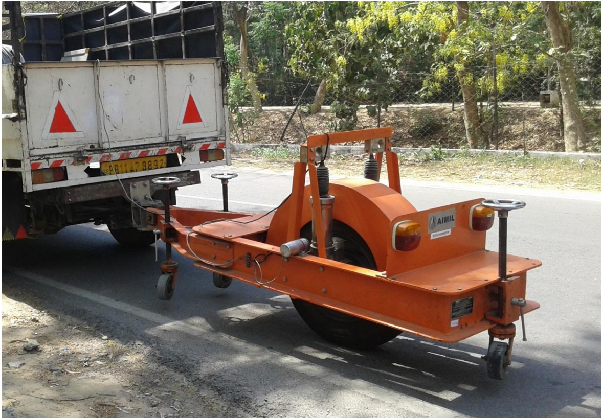
Figure 4.22: Bump Integrator (Roughometer) Towed with Pick-up
