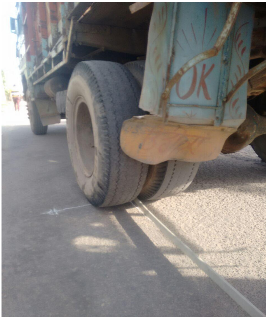
Figure 4.9: Placement of Beam Probe in between Rear Tyres of Truck
