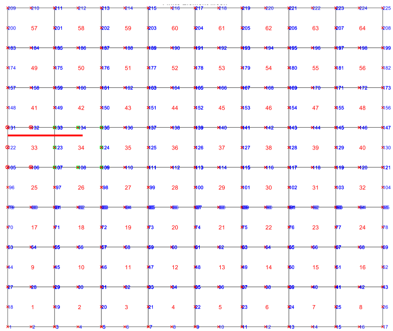
Fig. 3-7: FG-CNTRC plate with pre-existing crack modelled in the framework of XFEM indicating standard element, split element, and tip elements
