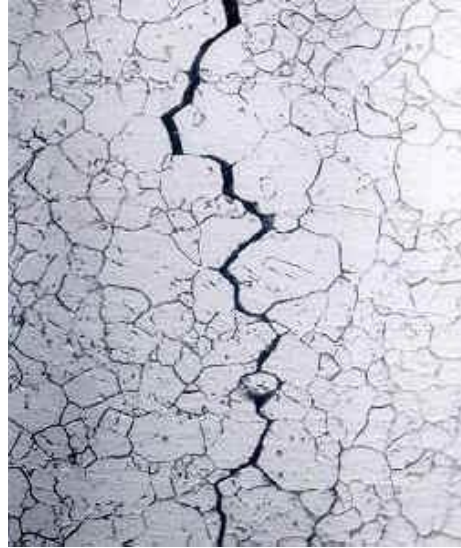
Figure 1.8 Stress corrosion cracking [17]
