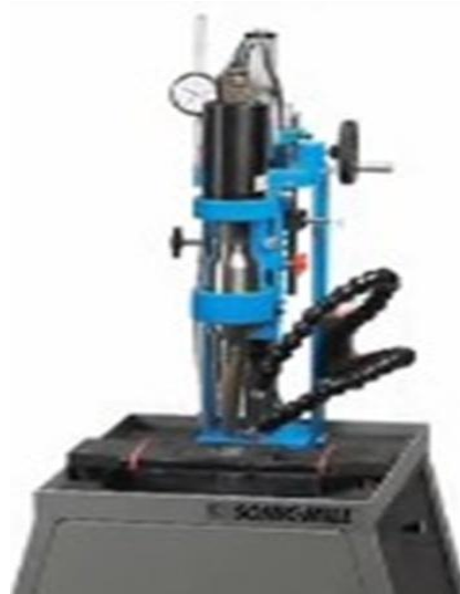
Figure 3.7 Ultrasonic machining setup (Type: Sonic Mill, USA)
