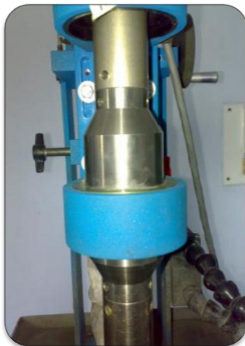
Figure 3.4 Ultrasonic transducer for compact 500W ultrasonic machine
