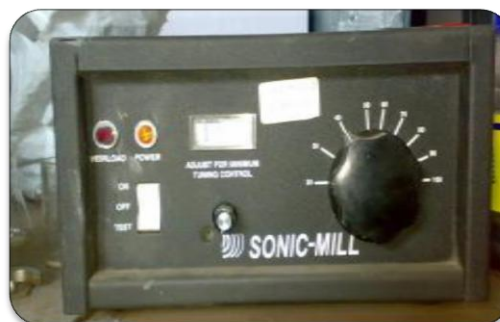
Figure 3.6 Power rating set-up for ultrasonic machine
