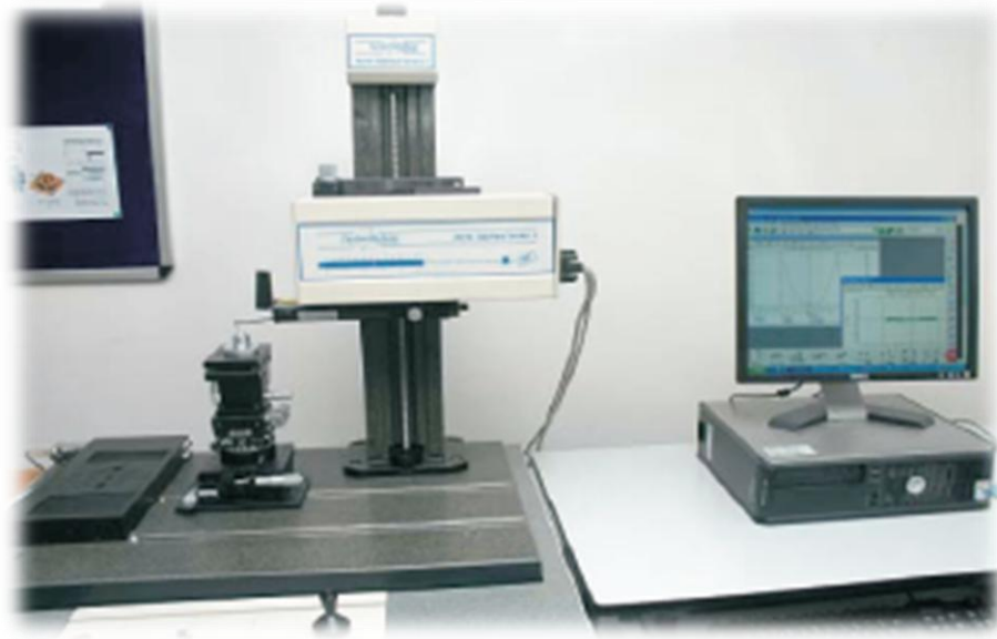
Fig 3.9: Contact Profilometer PGI 120 (Taylor Hobson Make)
