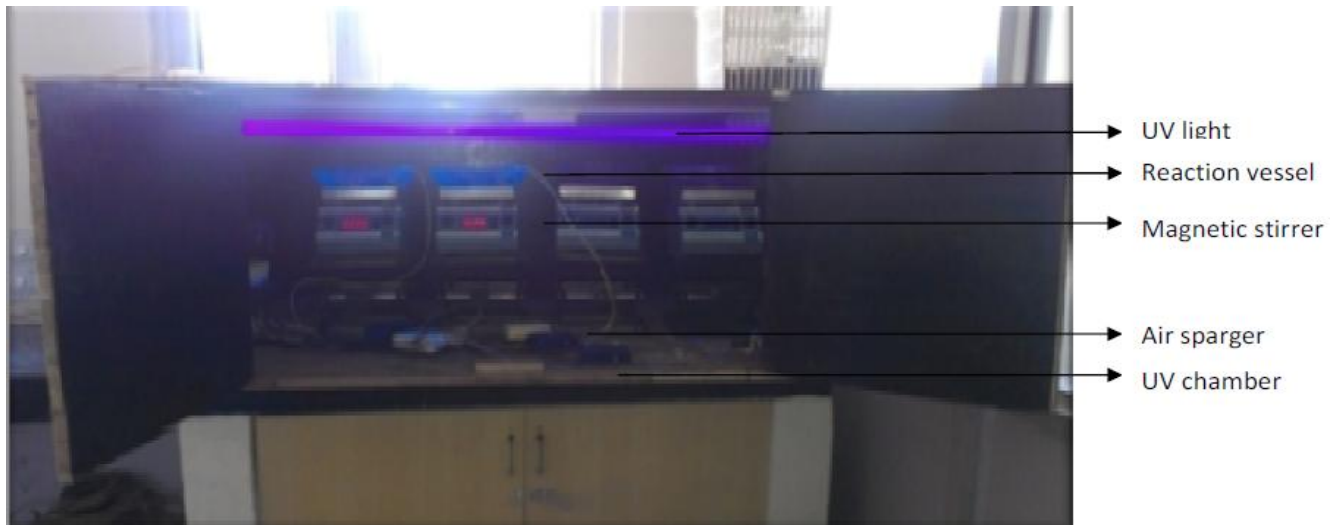
Figure 4.2 Photo reactor at lab scale during photocatalytic treatment
