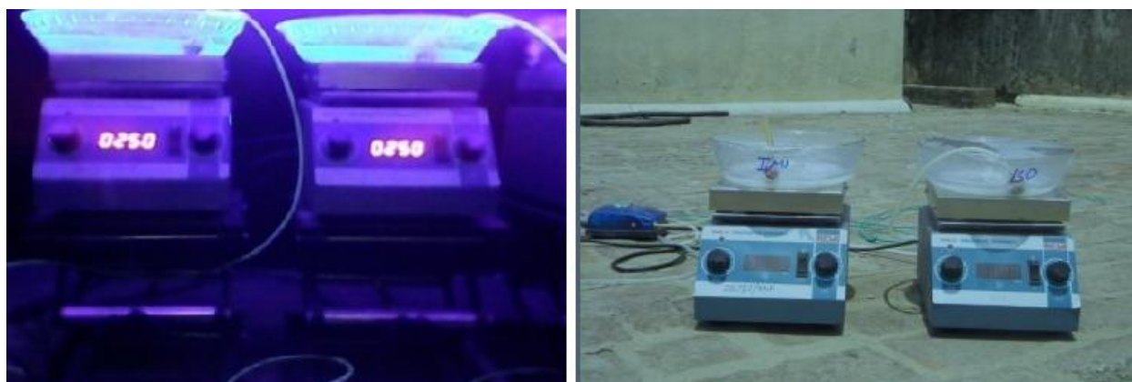
Fig (5.4) Small pond glass reactor vessel in (a) UV light (b) solar light
