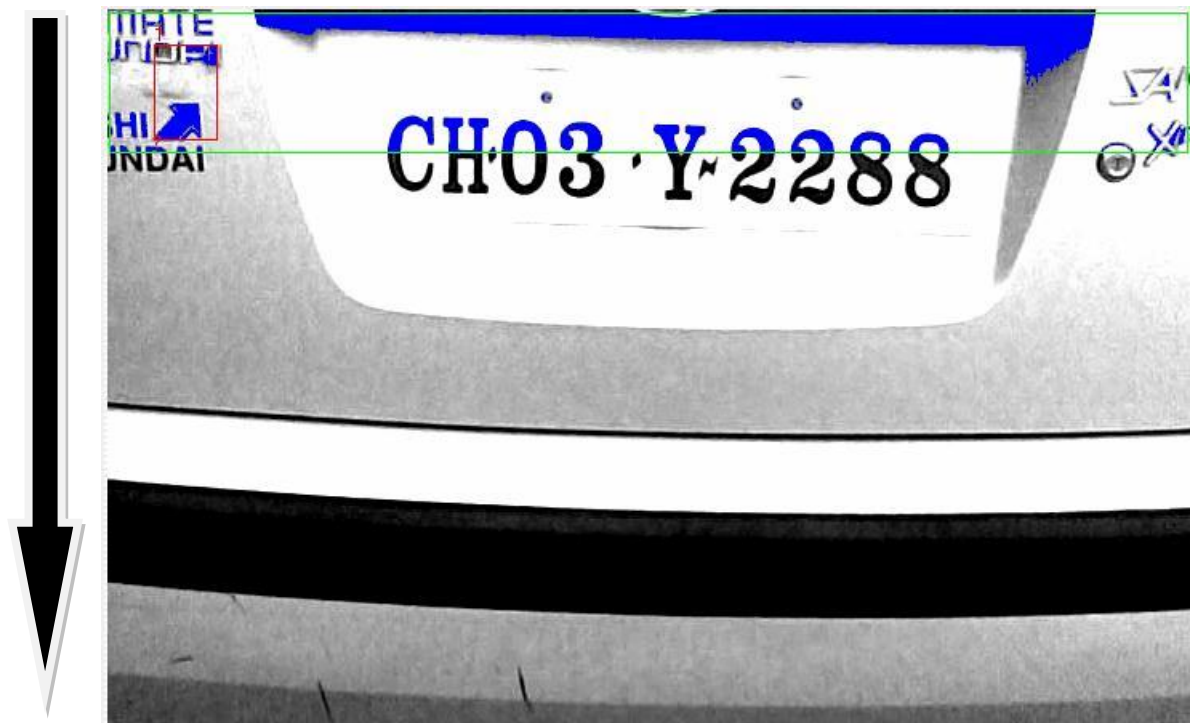
Fig 5.7 Bounding box specified by ROI descriptor, searching for number plate
