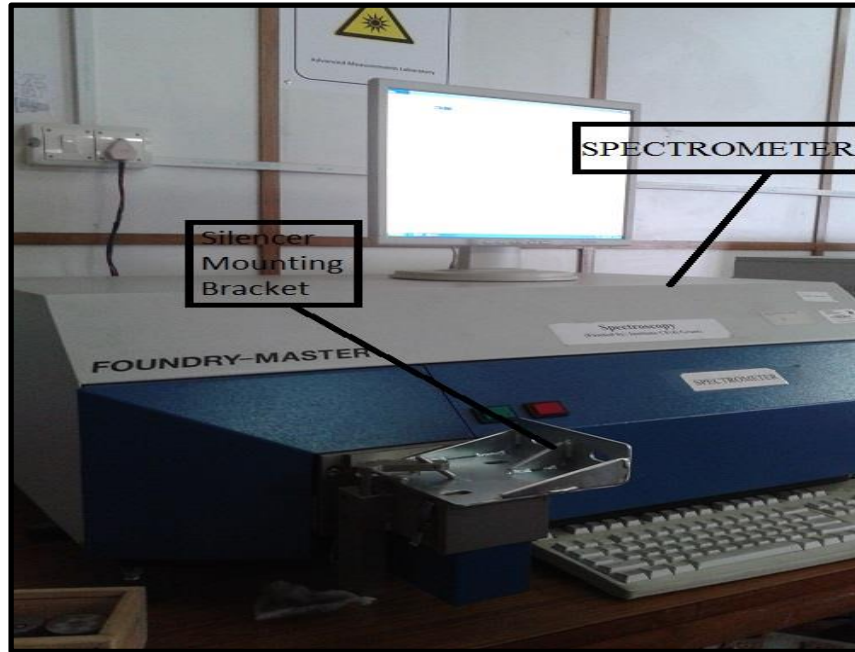
Figure 3.2 Spectrometer Used for Spectroscopy of silencer mounting bracket
