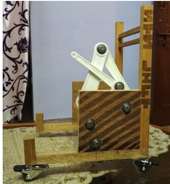
Fig. 6.2 Scaled Prototype of Assistive Device Incorporating (a) Primary Mechanism (b) Primary and Secondary Mechanism along Castor Wheels
