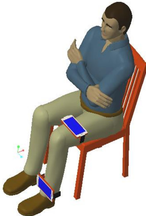
Fig. 3.9 Description of Attachment of Smartphones on Lower Limbs using PTC Creo Manikin [27]
