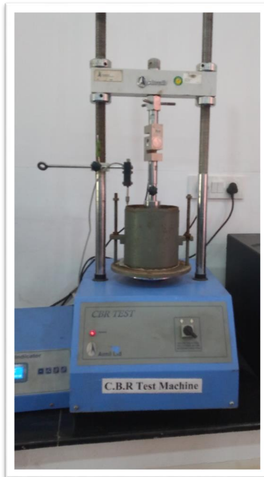
Figure 3.8: Testing of the sample after 96 hours in CBR test machine
