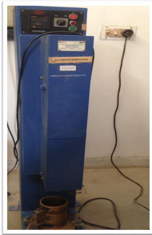
Figure 3.7: Automatic compactor used for proctor compaction test
