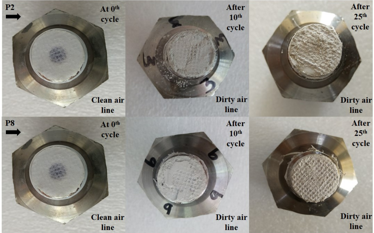
Figure 2.2: Pictorial representation of transducers showing filter conditions after 0th (before the start of conveying), 10 th and 25 th conveying cycles installed in P2 and P8 locations
