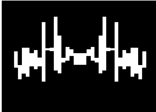
Figure.2.6: Optimized Antenna Design for Chip Impedance of 15-j250\Omega [10].
