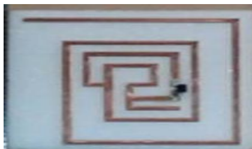
Figure 2.4: Fabricated Spiral RFID Tag Antenna[12].
