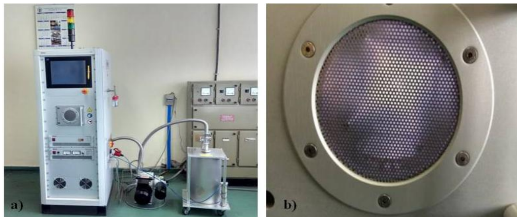
Figure 7: (a) Low Pressure Plasma reactor PICO (b) Plasma chamber
