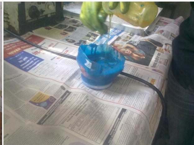
Fig. 4.11 Mixing of Epoxy and Hardener
