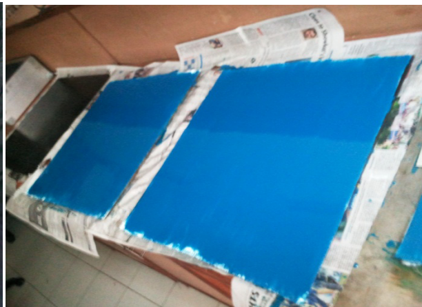
Fig 4.13 After resin application
