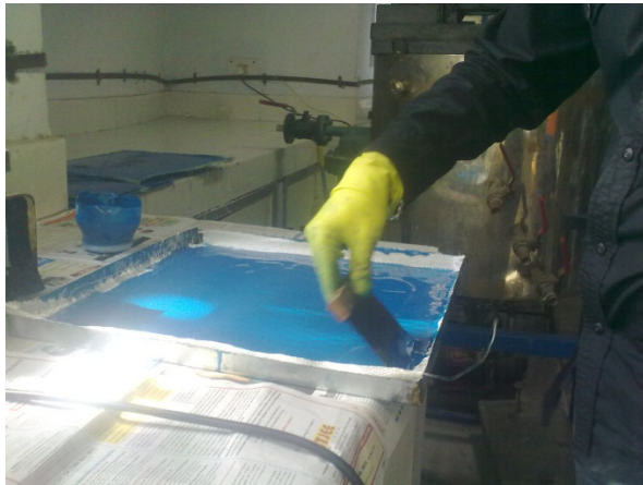
Fig 4.12 Applying resin on sheet
