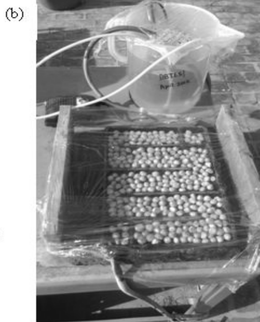
Figure 6.12(a). Degradation studies of Cephalexin using pilot-scale fixed-bed reactor with recirculation (b) Actual photo of pilot-scale solar fixed-bed reactor.
