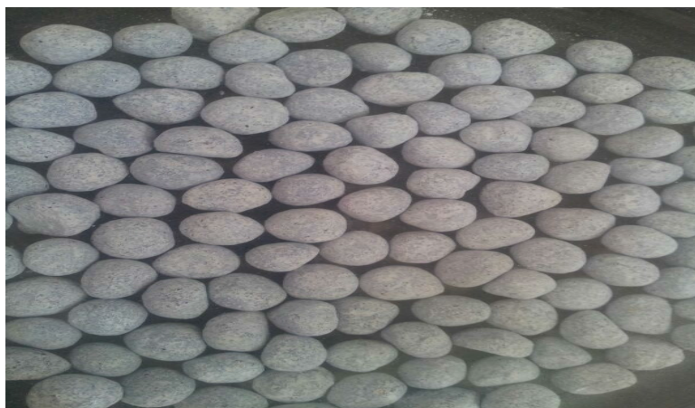
Figure 5.3: TiO 2 coated cement beads.
