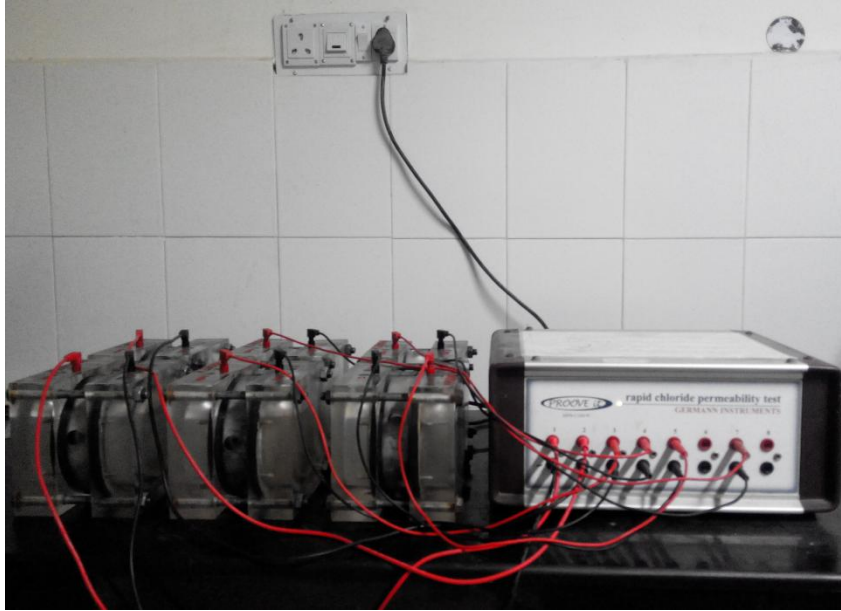
Fig 3.4 Rapid Chloride Permeability Test
