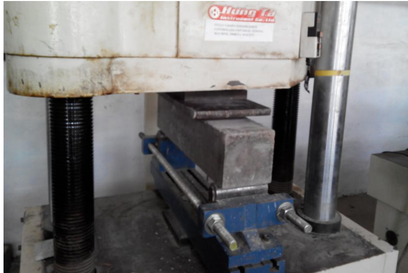
Fig.3.2 Testing of concrete beams in flexure
