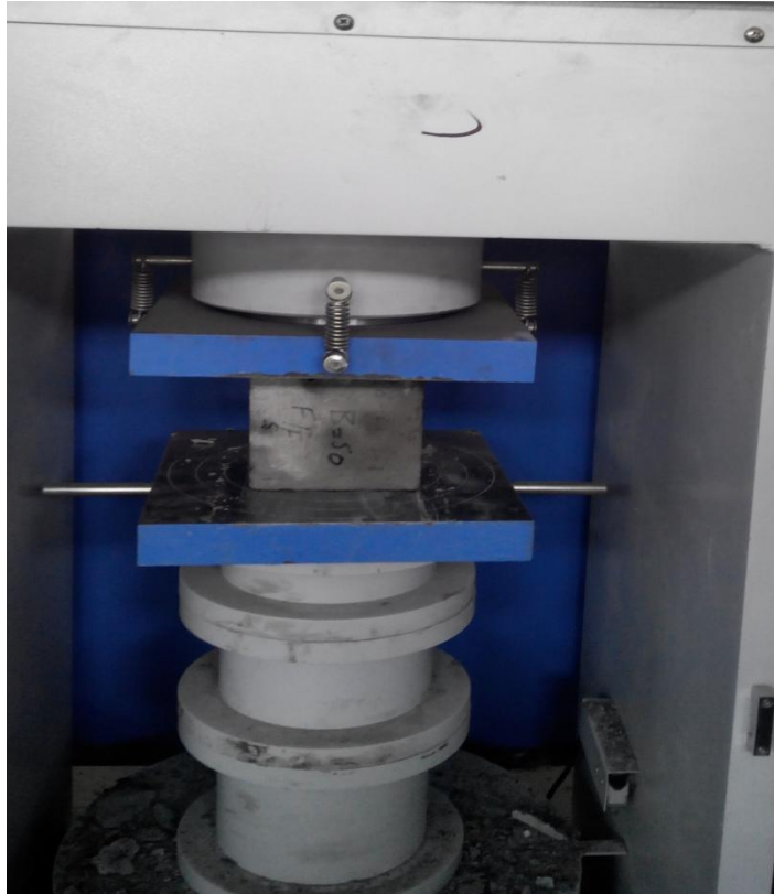
Fig.3.1 Testing of concrete cubes for compressive strength
