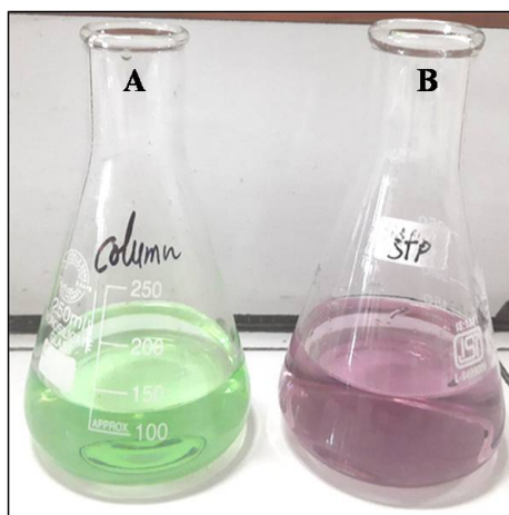
Figure 3.7: Change in colour of mixed indicator before and after titration
