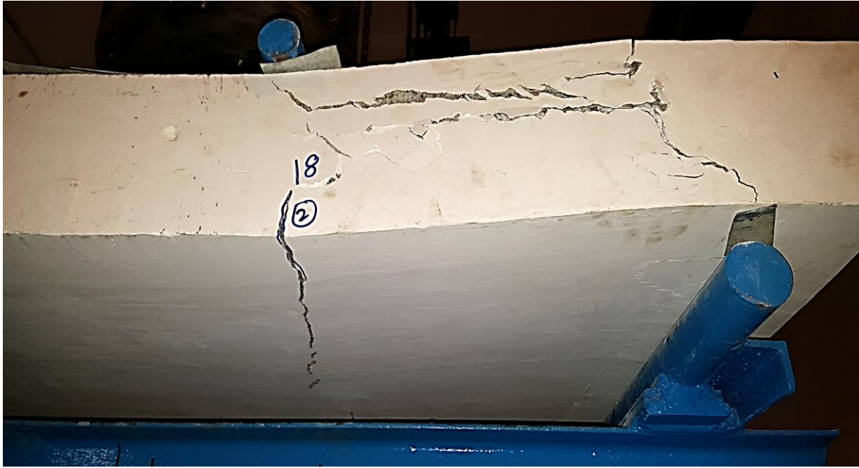
Figure 4. 3: Cracks are observed under the loading point throughout the width of the specimen.
