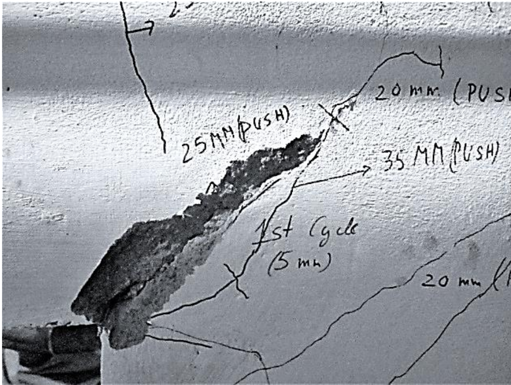
Figure 5. 12: Spread of cracks from opening corner to corner of frame
