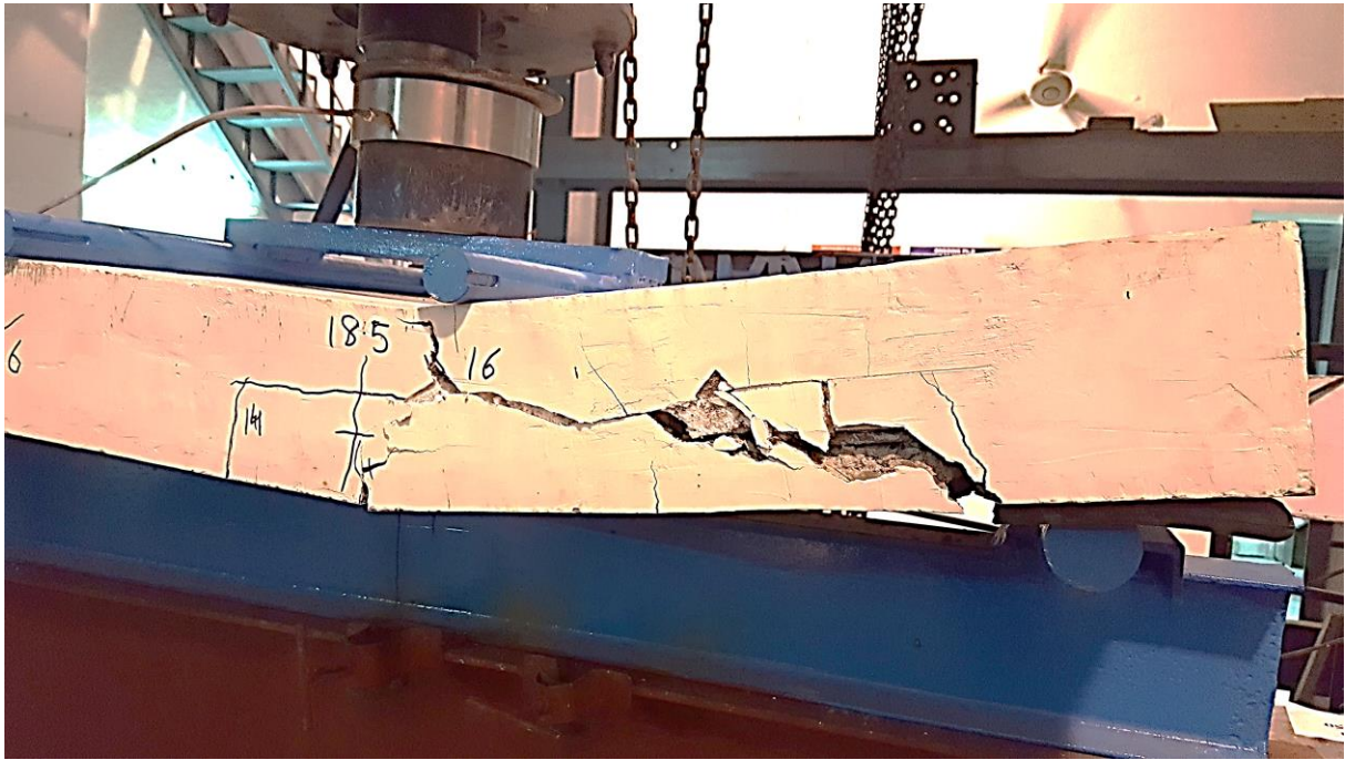
Figure 4. 1: Failure of specimen SPC1 at one of the loading points
