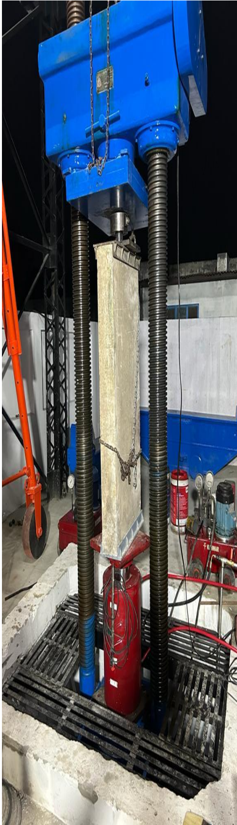
Figure 3. 32: Test setup for axial compression testing with load cell attached the top.
