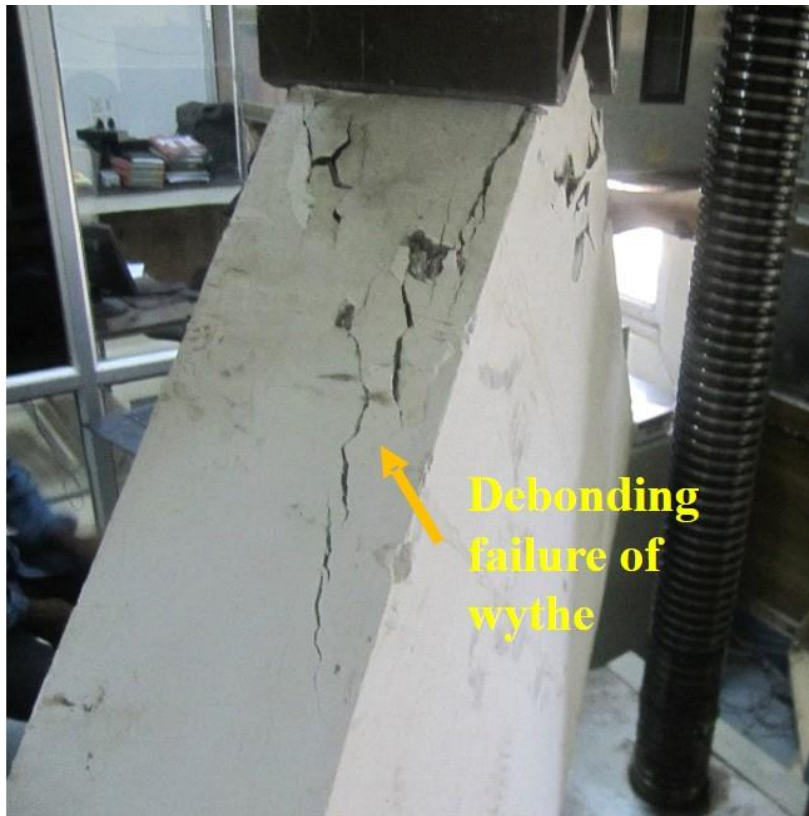
Figure 4. 24: Debonding failure of specimen DS1Sgi300
