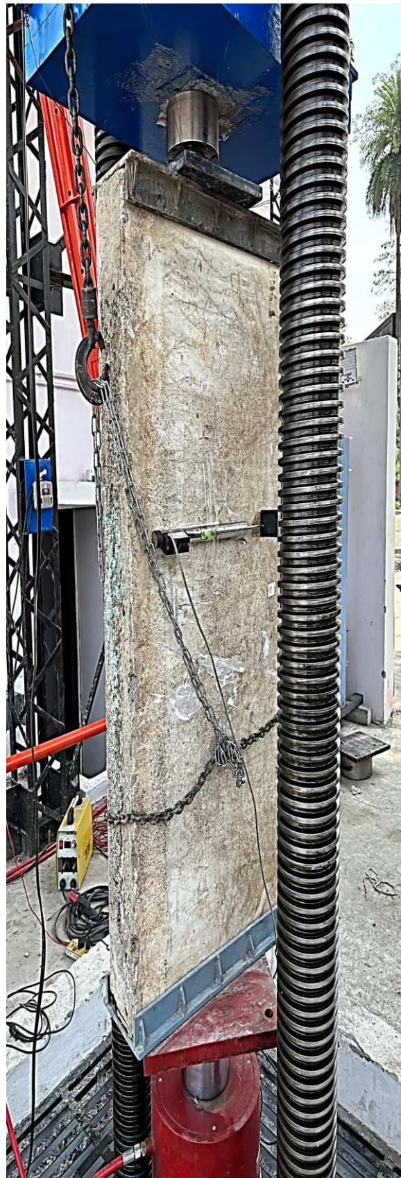
Figure 3. 32: Test setup for axial compression testing with load cell attached the top.
