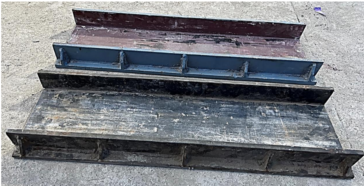
Figure 3. 31: Steel shoes for testing of CSP in axial compression
