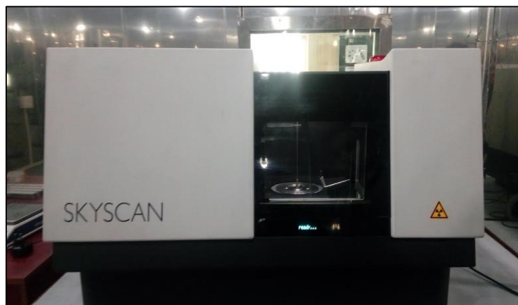
Figure 4.22: Schematic diagram of microcomputer tomography machine.
