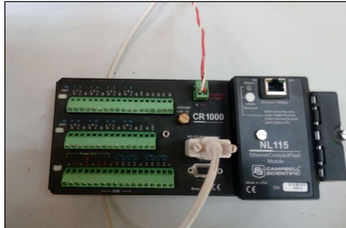
Figure 3.13: Data logger CR1000.
