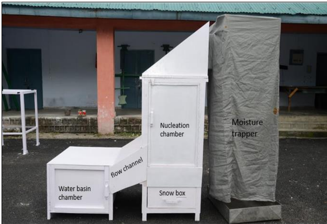
Figure 3.4: Wooden prototype of artificial snow making machine.
