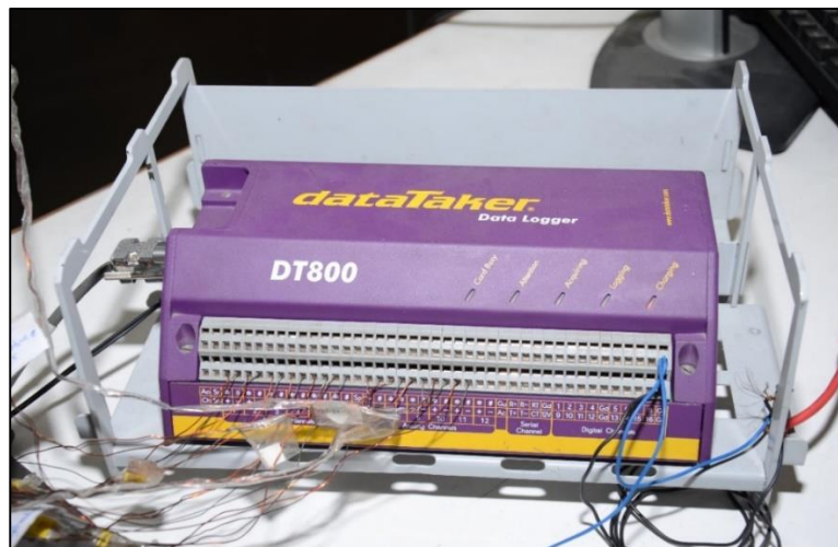
Figure 3.12: Data acquisition by data Taker DT800.
