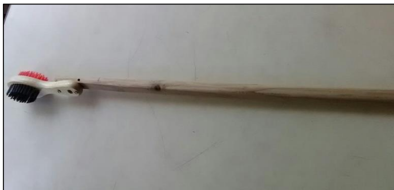
Figure 3.7: Brush for harvesting the snow from the nylon wire into snow box.
