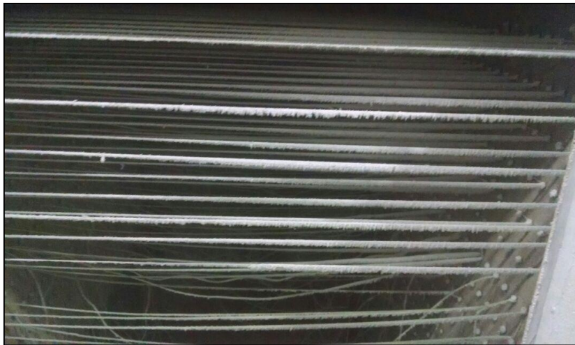
Figure 3.5: Growth of snow crystals on the nylon wires after the first experiment
