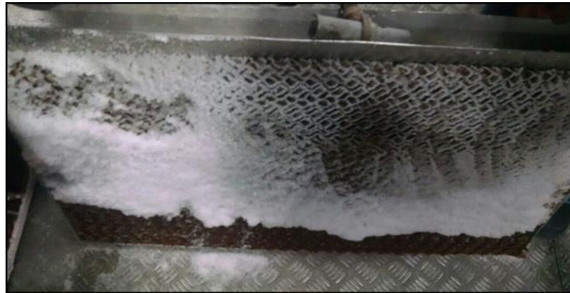
Figure 3.6: Deposition of snow on the front side of the honeycomb mesh.
