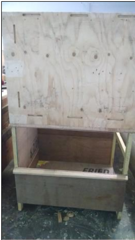
Figure 3.2: Snapshot of nucleation chamber of snow making machine.
