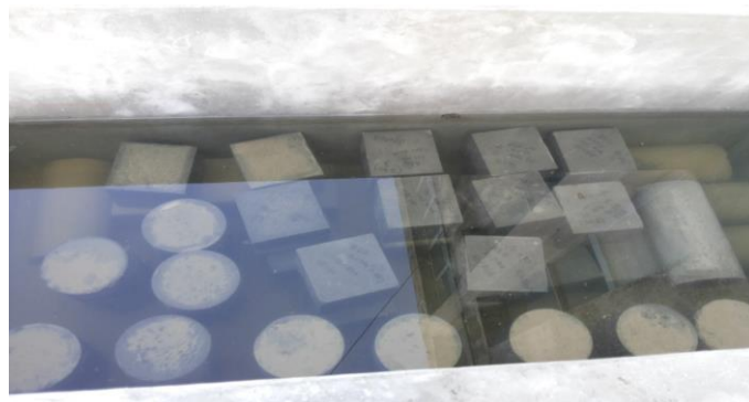
Fig 3.9: Curing of SCC specimens
