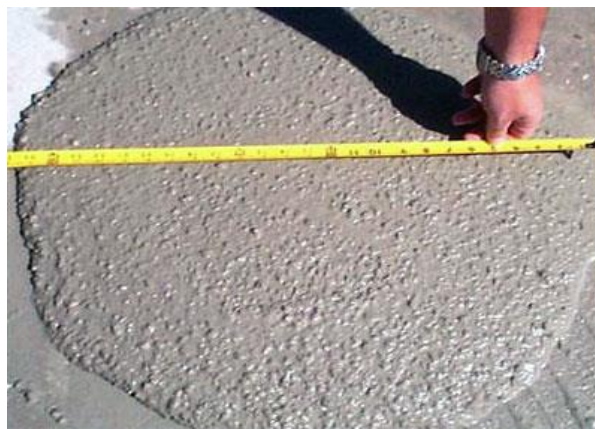
Fig 3.10: Slump flow test for SCC
