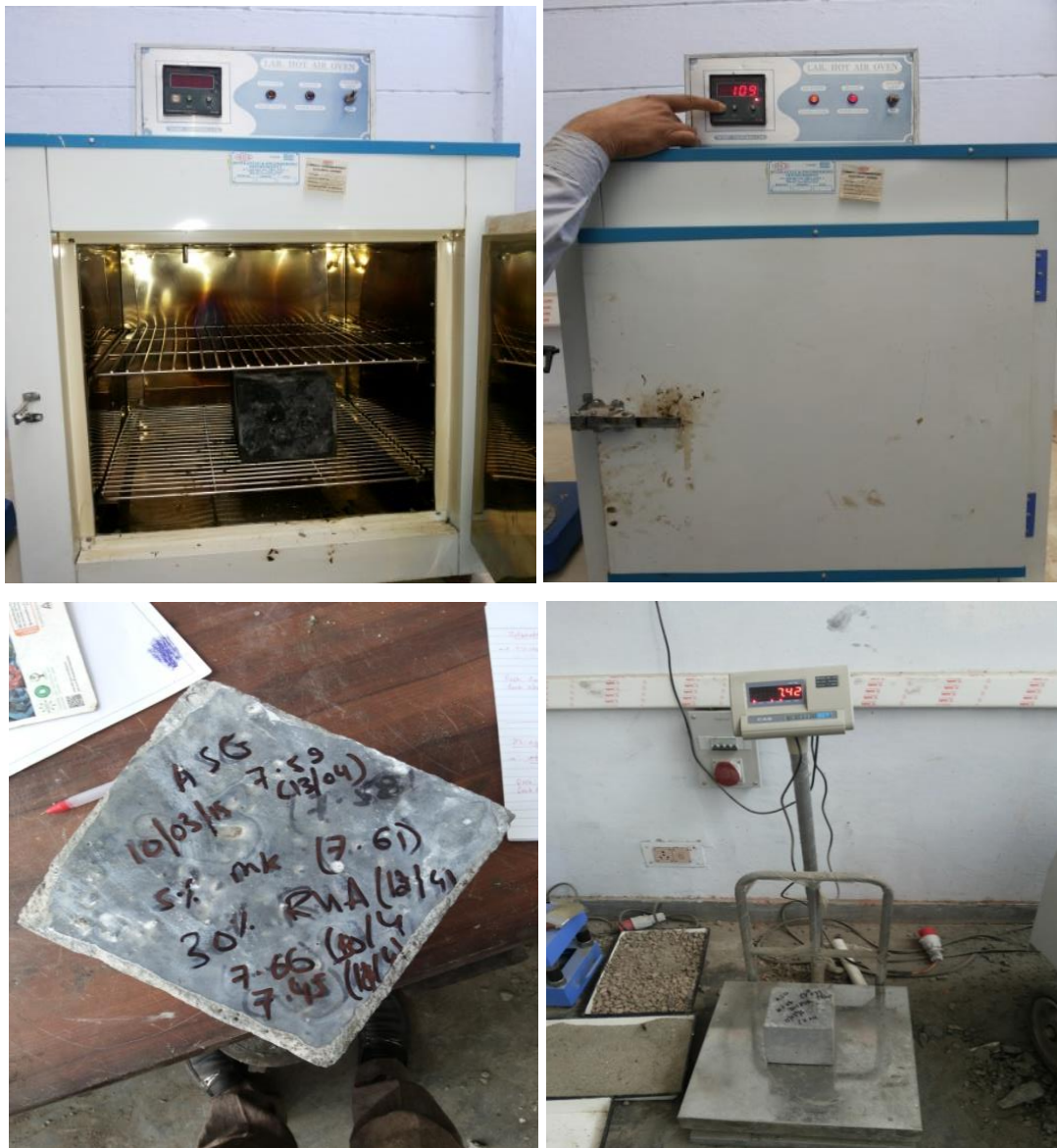
Fig 3.17: Water absorption test in progress
