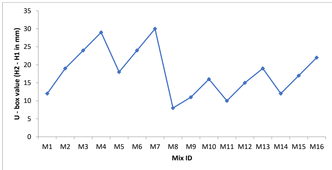
Fig 4.5: Comparison of U – box values of all SCC mixes
