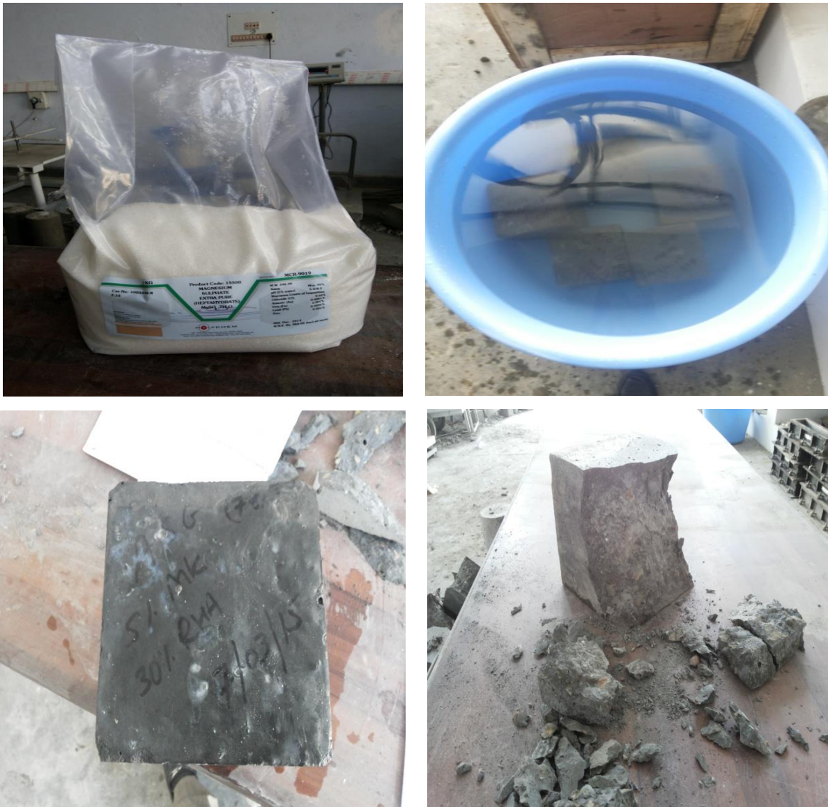
Fig 3.18: (a) Magnesium sulphate in powder form, (b) specimens immersed in magnesium sulphate solution, (c) specimen after 90 days of immersion in magnesium sulphate solution, (d) specimen after tested for compressive strength.
