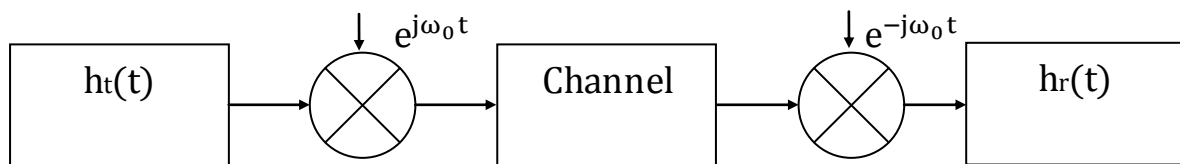
Figure 21: Basic structure of a single carrier system.
