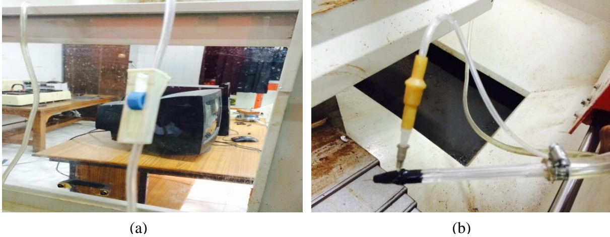
Figure 3.10: (a) Coolant controller (b) Coolant outlet pipe connected to Tapered nozzle
