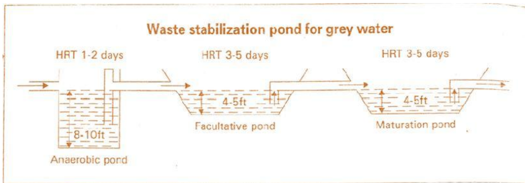
Fig.3.1 Waste Stabilization Pond for Grey Water
